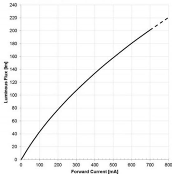
**Figure 2. Forward Current as a Function of Applied Voltage and Its Effect on Luminous Flux Output**
