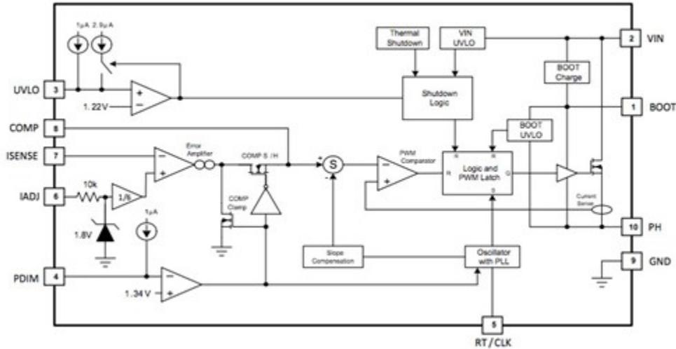
**Figure 5. Functional Block Diagram of the TPS92512**
