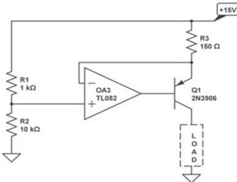
**Figure 4. A High Side Current Control Circuit Using an Op-amp**
