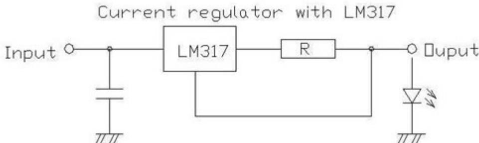
**Figure 3. Circuit Diagram for an LM317 Based Constant Current Source**
