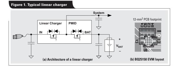
During normal operation with an input present, the first switch turns on and shorts the input to PMID, while the second switch modulates its resistance in order to regulate the current and voltage at the battery output.
