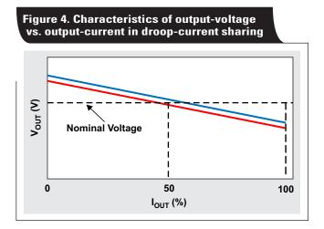
The bigger the k, the more accurate the current sharing, but the more deviation of output voltage versus load.
