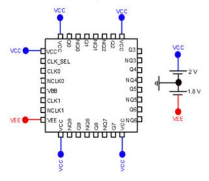
Figure 3-1. Bias Diagram Used in TID Exposure
