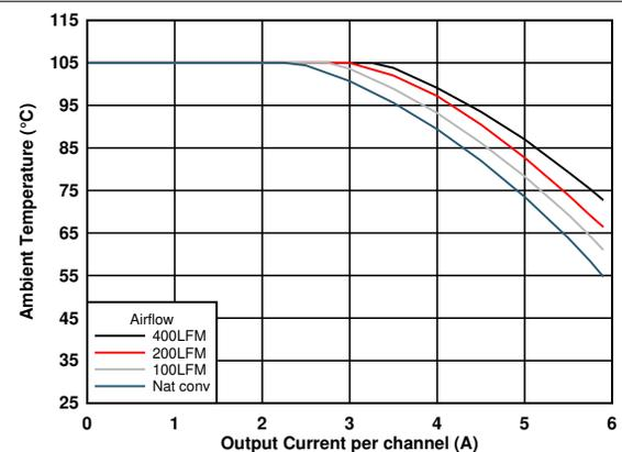
Fsw = 2.0 MHz Dual 3.3-V outputs IOUT1 = IOUT2
