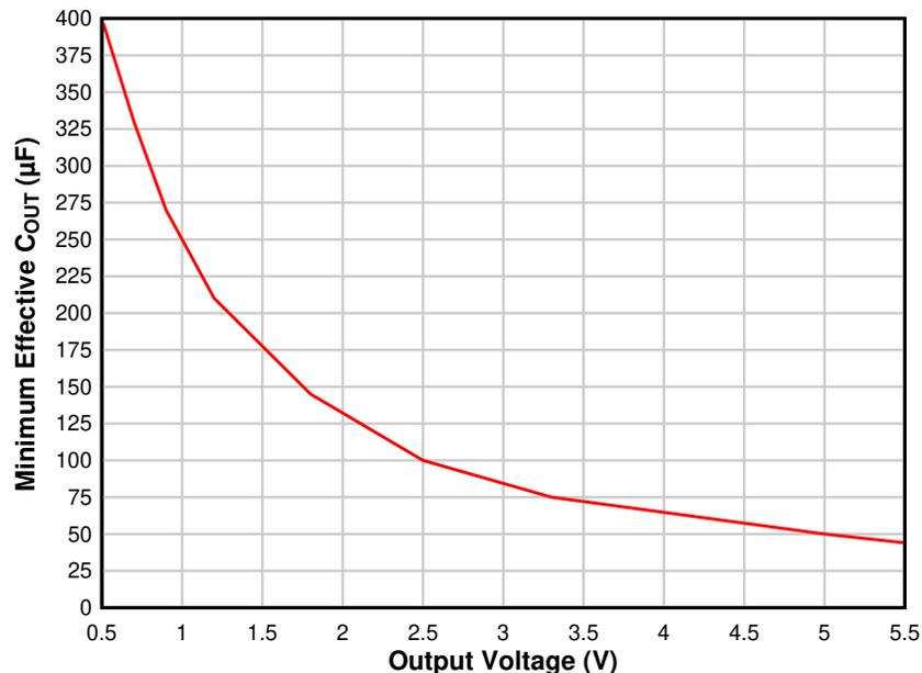
图 7-5. Minimum Required Output Capacitance (per Phase)
