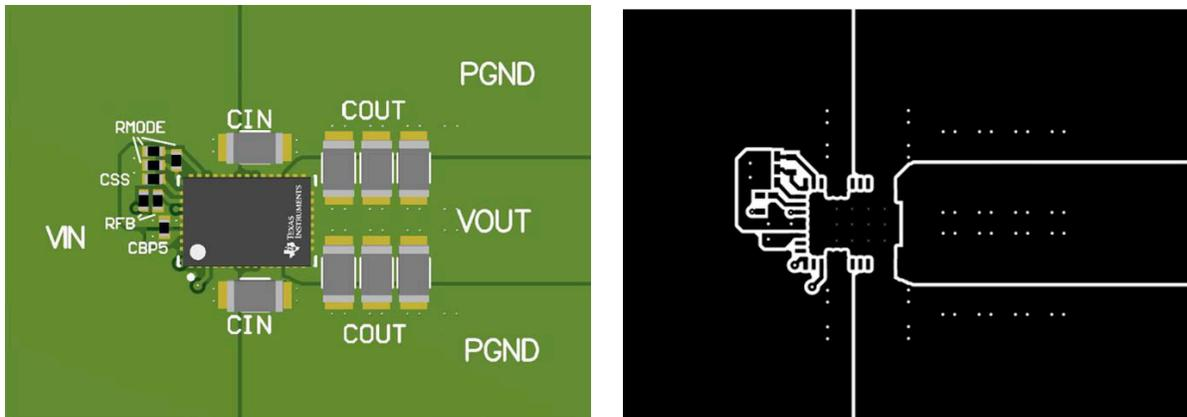
图 10-2. Typical Parallel-Output Layout
