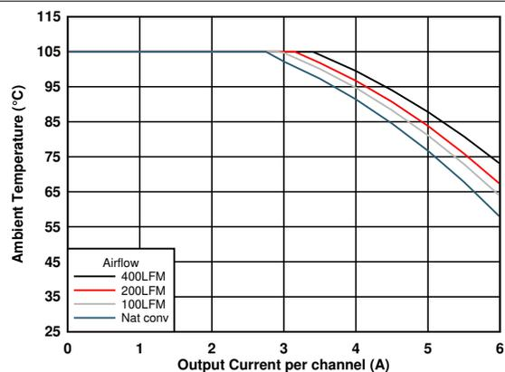
Fsw = 1.5 MHz Dual 1.8-V outputs IOUT1 = IOUT2
