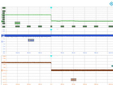
Ch2: Output voltage (4 V/div); Ch3: LED current (1 A/div);
