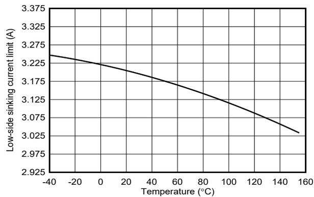
Figure 5-5. Low-Side Sinking Current Limit vs Temperature
