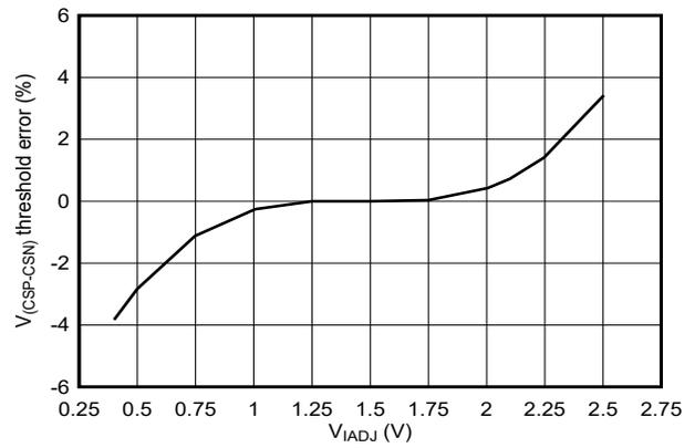
**Figure 5-8.  $V_{(CSP-CSN)}$  Sense Error vs IADJ Setpoint**
