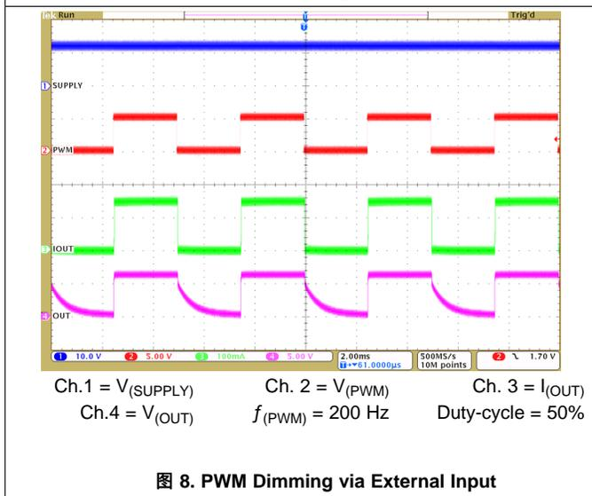
图 8. PWM Dimming via External Input
