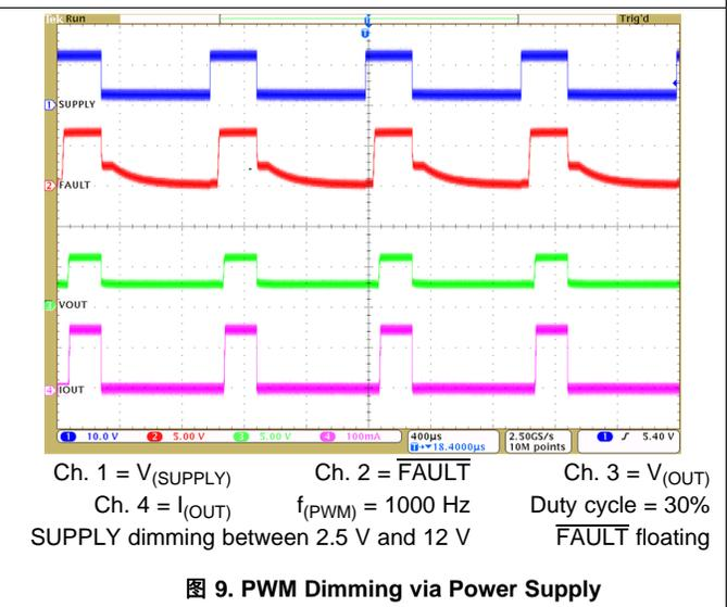
图 9. PWM Dimming via Power Supply
