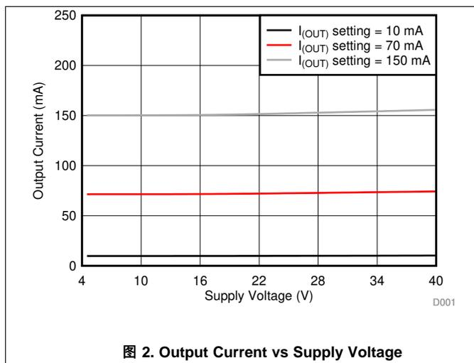
图 2. Output Current vs Supply Voltage
