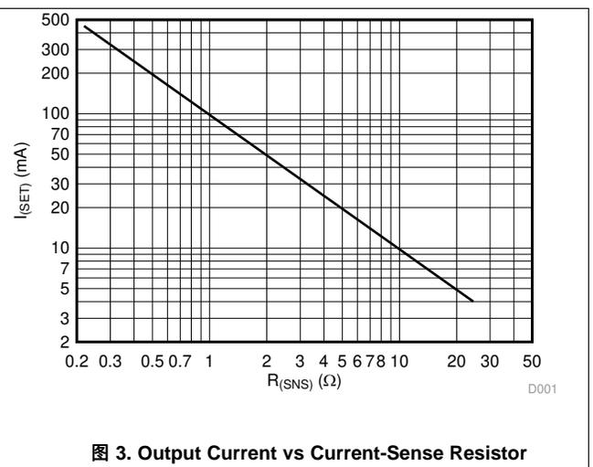
图 3. Output Current vs Current-Sense Resistor
