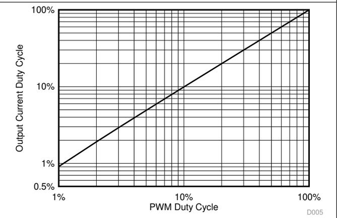
图 7. PWM Output Duty Cycle vs Input Duty Cycle
