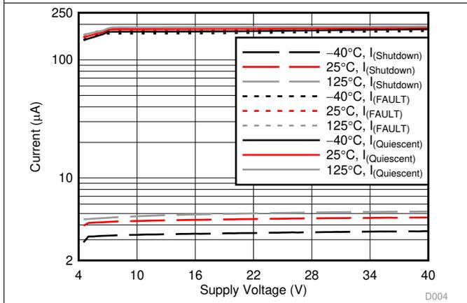
图 6. Shutdown, Quiescent, and Fault Current vs Supply Voltage
