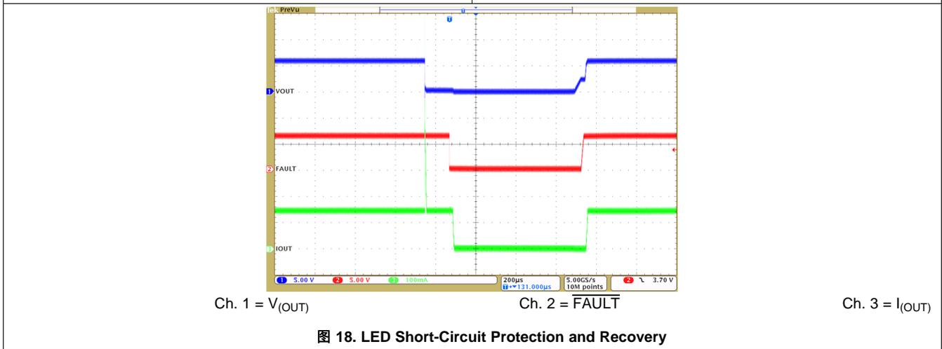
图 18. LED Short-Circuit Protection and Recovery
