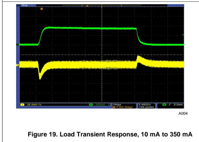
Figure 19. Load Transient Response, 10 mA to 350 mA
