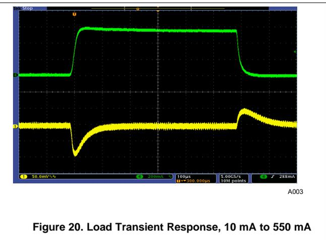
Figure 20. Load Transient Response, 10 mA to 550 mA
