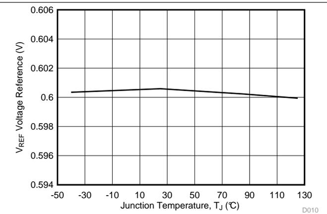
Figure 10. Voltage Reference vs Temperature
