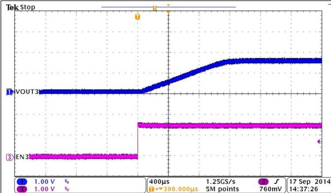
Figure 36. Buck3, Soft-Start, Iout = 2 A
