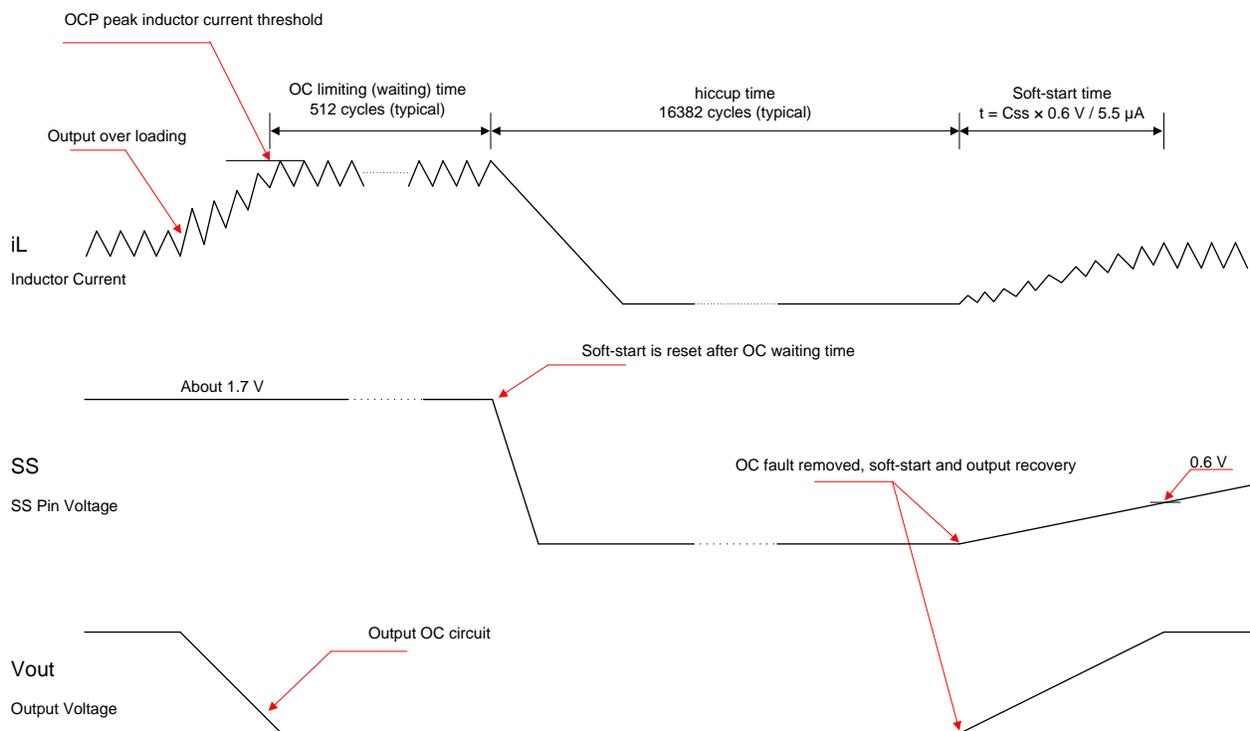
**Figure 29. Overcurrent Protection**
