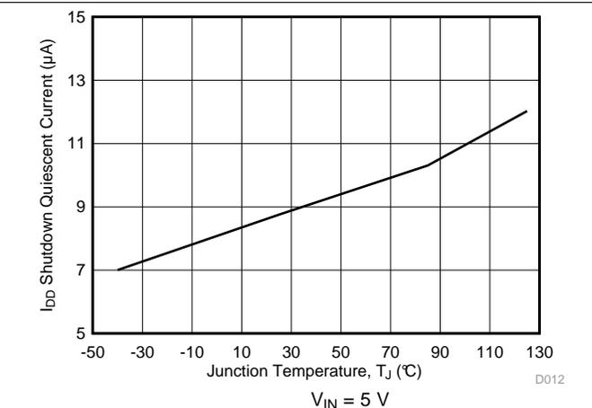
Figure 12. Shutdown Quiescent Current vs Temperature
