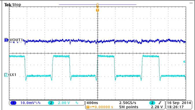
Figure 37. Buck1, Output Voltage Ripple, Iout = 3 A
