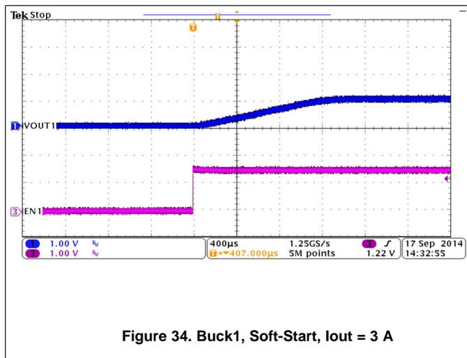
Figure 34. Buck1, Soft-Start, Iout = 3 A
