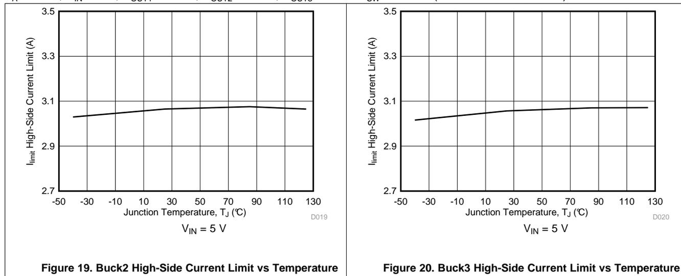
**Figure 19. Buck2 High-Side Current Limit vs Temperature**
