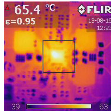
图 8-34. Thermal Signature of TPS65262EVM EVM Condition 4 Layers, 64 mm × 69 mm, T A = 30.5°C
