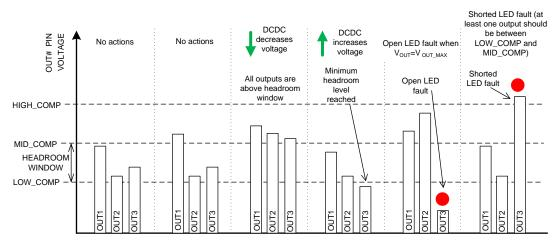
Figure 12. Protection and DC-DC Voltage Adaptation Algorithms
