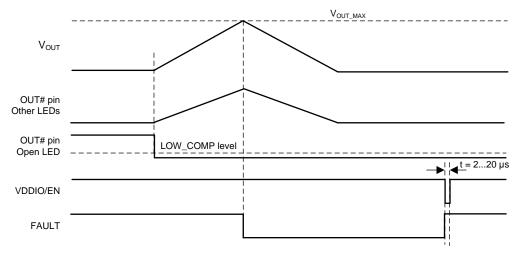
Figure 16. LED Open Fault
