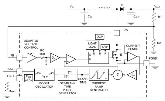
Figure 10. Boost Block Diagram
