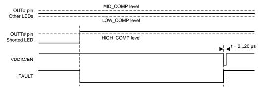
Figure 17. LED Short Fault
