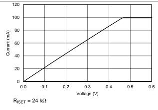
Figure 8. LED Current Sink Saturation Voltage
