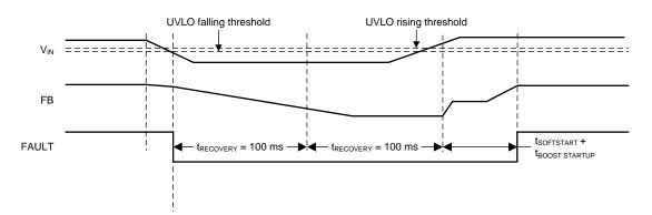
Figure 15. V<sub>IN</sub> Undervoltage Lockout
