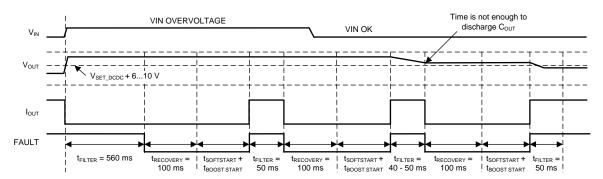
Figure 13. V<sub>IN</sub> Overvoltage Protection (DC-DC OVP)
