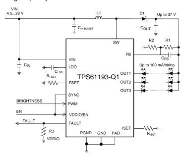
Figure 20. Three Strings 100 mA/String Configuration
