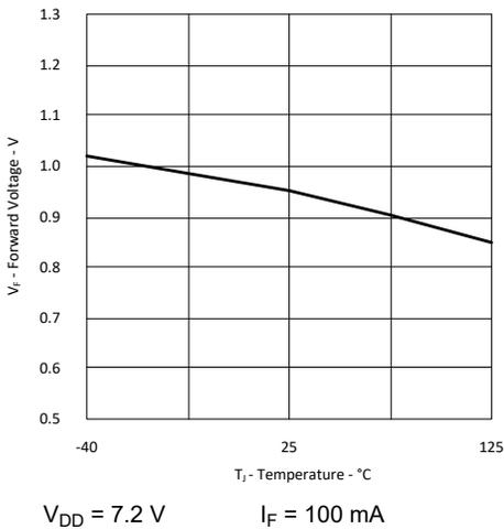
图 6-13. Bootstrap Diode Forward Voltage vs Temperature
