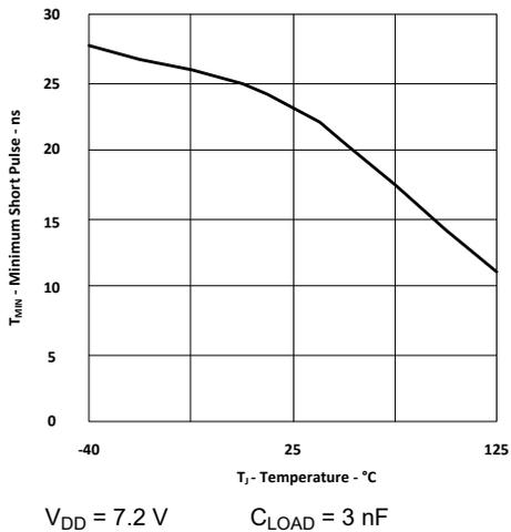
图 6-12. UGATE Minimum Short Pulse vs Temperature
