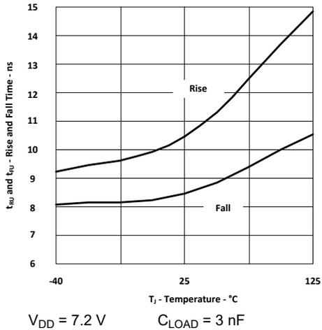
图 6-8. UGATE Rise and Fall Time vs Temperature
