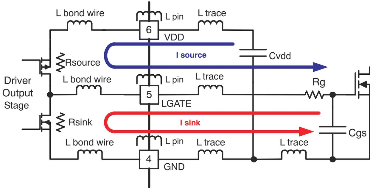
图 8-5. MOSFET Drive Paths and Main Circuit Parasitics
