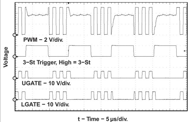
图 6-19. Normal and Three-State Operation ENTER/EXIT Conditions
