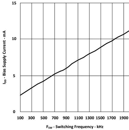
$V_{DD} = 7.2\text{ V}$  No Load  $T_J = 25^\circ\text{C}$
