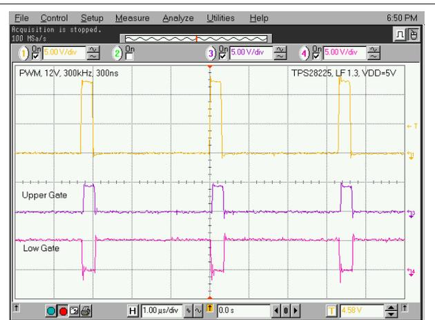
图 7-5. 12-V PWM Pulse at  $V_{DD} = 5$  V
