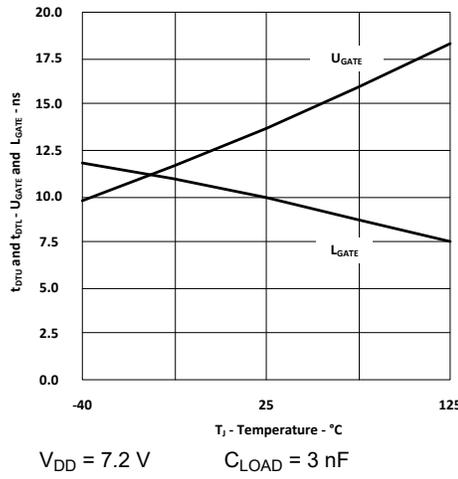
图 6-11. UGATE and LGATE (Dead Time) vs Temperature
