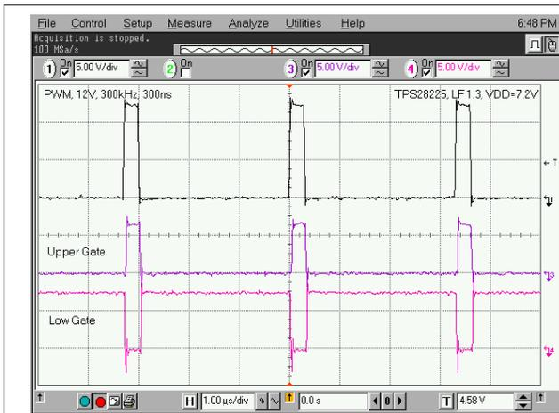
图 7-4. 12-V PWM Pulse at  $V_{DD} = 7.2$  V
