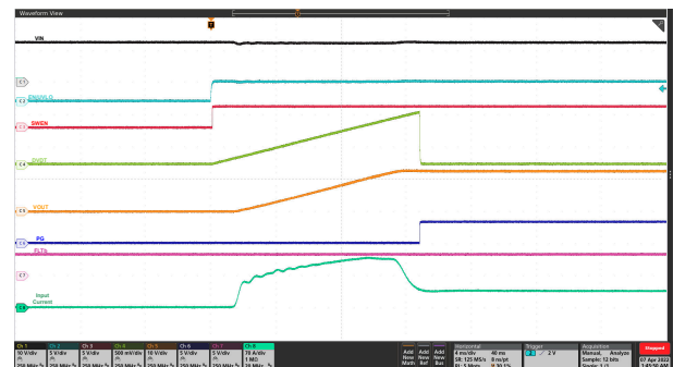
图 9-7. Start-up with EN/UVLO: V_{IN} = 12 V, EN/UVLO Stepped Up From 0 V to 3 V, C_{LOAD} = 50 mF, R_{LOAD(Start-up)} = 0.48 \Omega , C_{DVT} = 33 nF, and R_{ILIM} on Each Device = 442 \Omega
