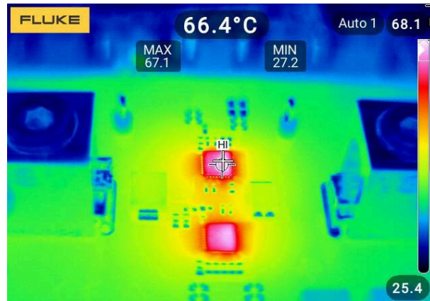
图 9-12. Two Devices in Parallel Temperature Rise with 110-A DC Current at Room Temperature (No Air-Flow)
