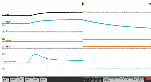
图 7-29. Input Overvoltage Protection Response
