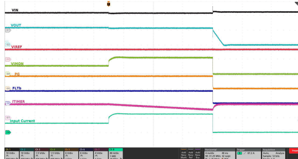
图 7-32. Overcurrent Protection Response (Circuit-Breaker)
