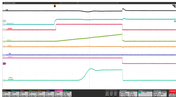
图 9-8. Power Up into Short: V_{IN} = 12 V, EN/UVLO Stepped Up From 0 V to 3 V, R_{REF} = 40.2 k \Omega , R_{ILIM} on Each Device = 442 \Omega , and OUT Shorted to GND
