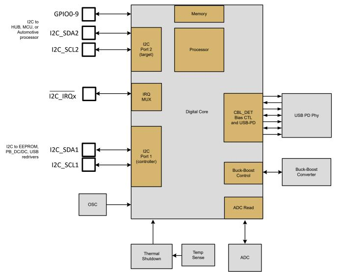
图 9-41. Digital Core Simplified Block Diagram
