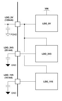
Note: LDO\_5V max regulation current includes LDO\_3V3 (25 mA) and LDO\_1V5 (10 mA)
