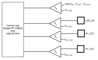
图 9-29. Over-voltage and Reverse Current Protection
