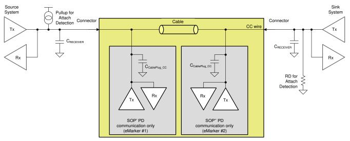
图 9-25. Example USB-PD Multi-Drop Configuration
