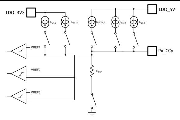
图 9-27. Plug and Orientation Detection Block
