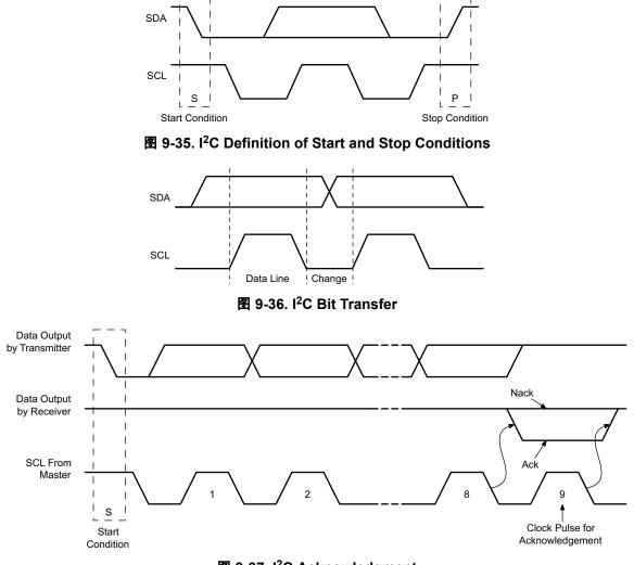
图 9-37. I<sup>2</sup>C Acknowledgment
