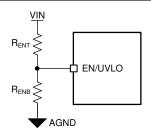
图 9-2. UVLO Threshold Programming
