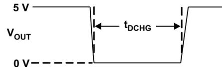
Figure 26. OUT Discharge During Mode Change
