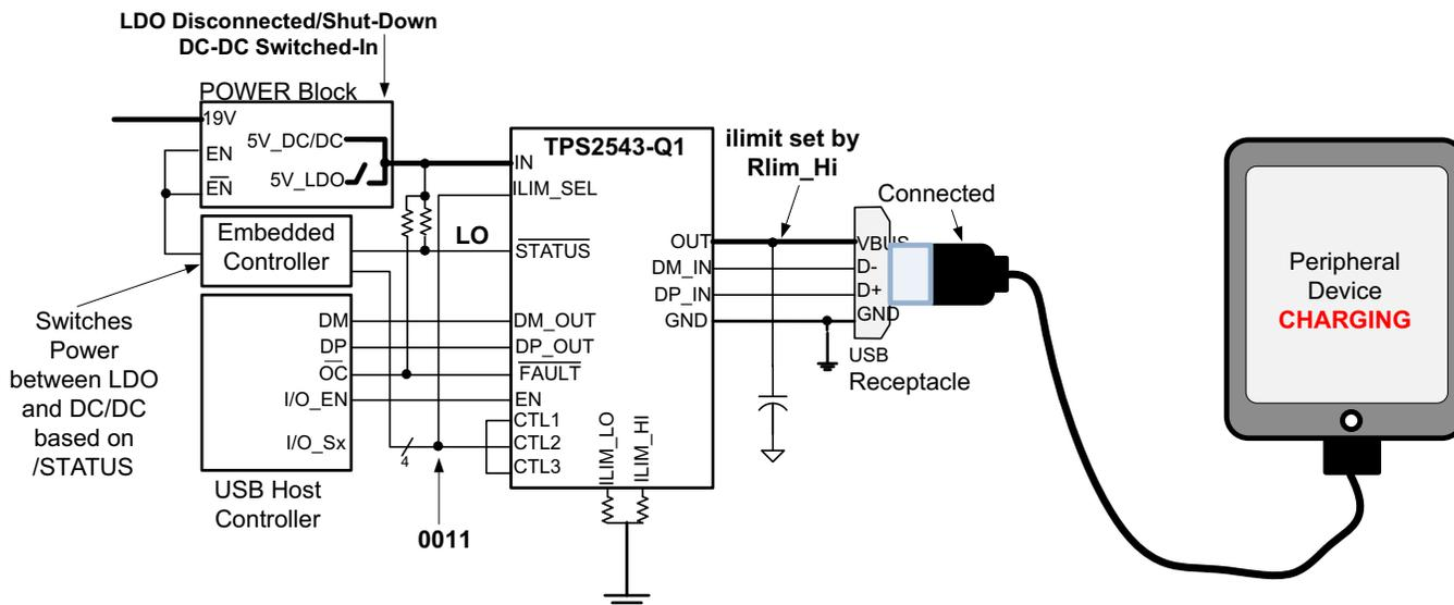
Figure 35. Case 1: System in S4/S5, Device Charging
