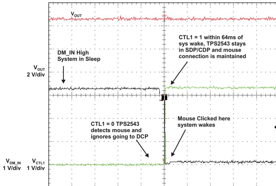
Figure 33. Mouse Wake from Sleep Scope Plot
