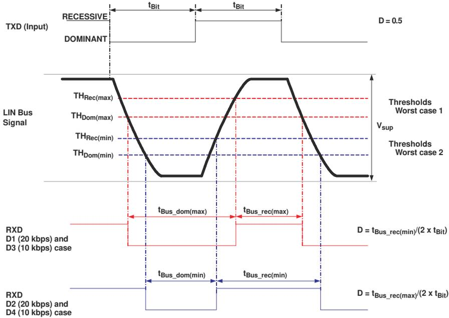
图 8-1. Definition of Bus Timing Parameters
