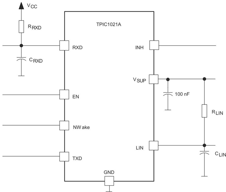
图 9-1. Test Circuit for AC Characteristics
