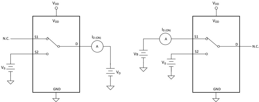
shows the circuit used for measuring the on-leakage current, denoted by  $I_{S(ON)}$  or  $I_{D(ON)}$ .
