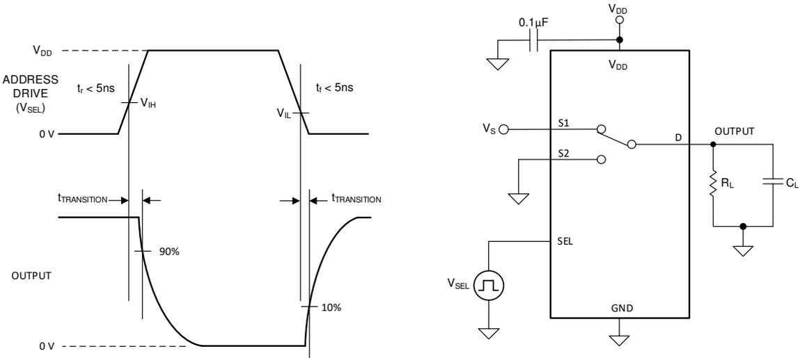
shows the setup used to measure transition time, denoted by the symbol  $t_{TRANSITION}$ .
