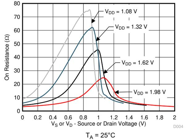
图 5-4. On-Resistance vs Source or Drain Voltage
