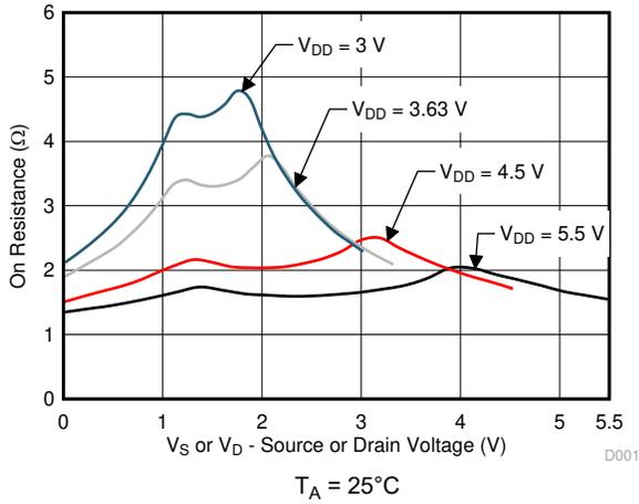
图 5-1. On-Resistance vs Source or Drain Voltage
