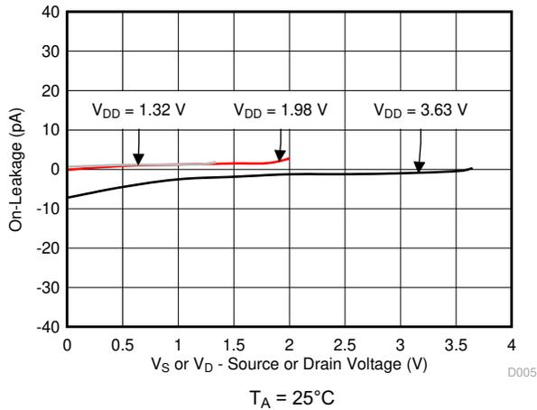
图 5-5. On-Leakage vs Source or Drain Voltage
