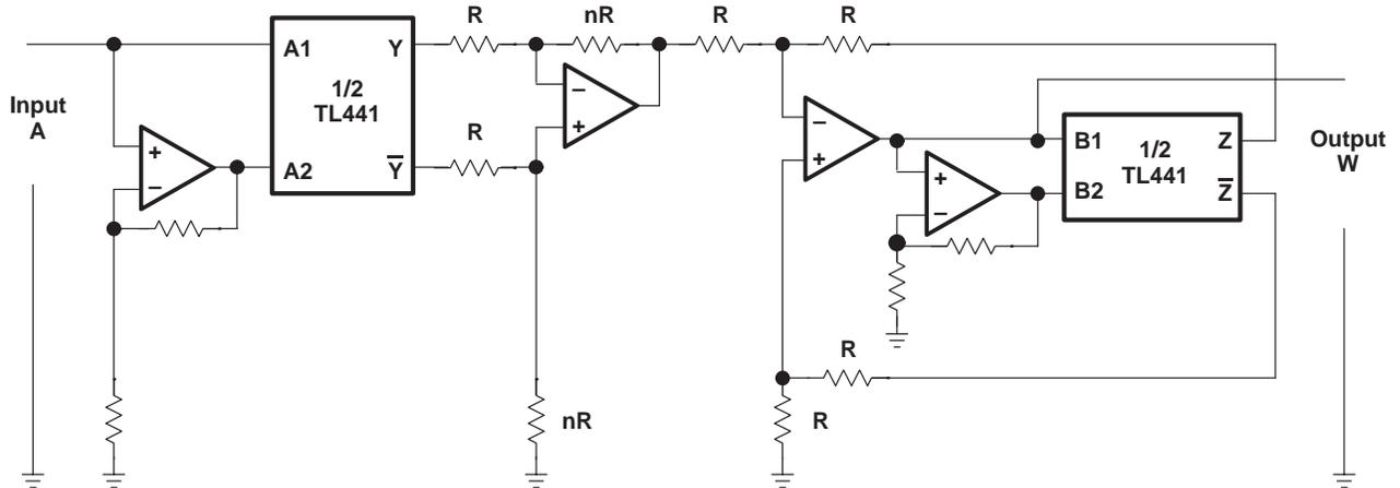
NOTE: R designates resistors of equal value, typically 2 kΩ to 10 kΩ. The power to which the input variable is raised is fixed by setting nR. Output W may need to be amplified to give the correct value.
