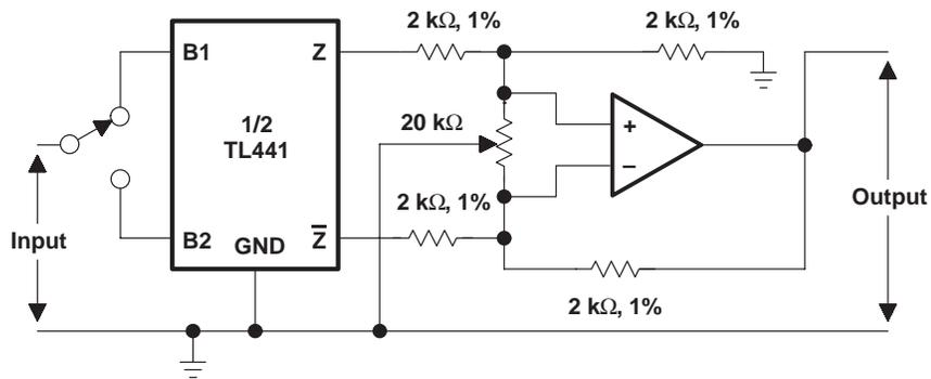
Figure 13. Utilization of Separate Stages
