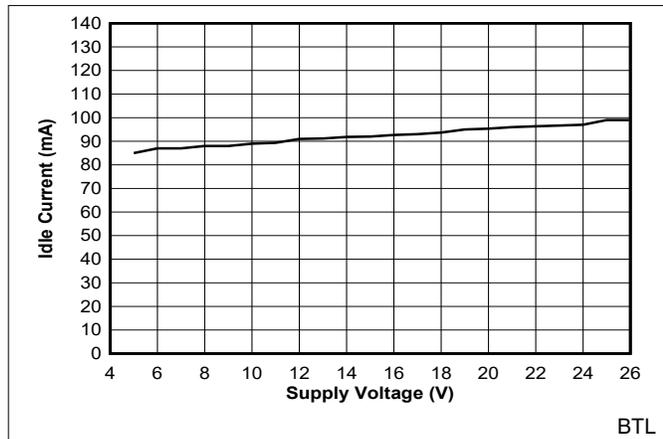
图 7-13. VBAT Idle Current vs Supply Voltage
