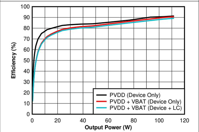
图 7-6. Efficiency vs Output Power - 14.4 V - 4 Ohm
