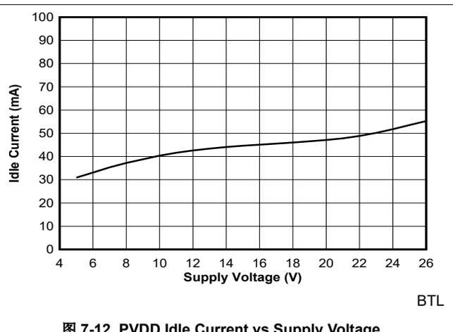
图 7-12. PVDD Idle Current vs Supply Voltage
