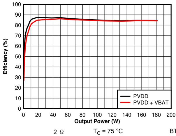
图 7-25. Efficiency vs Output Power - 2  $\Omega$  - 384 kHz
