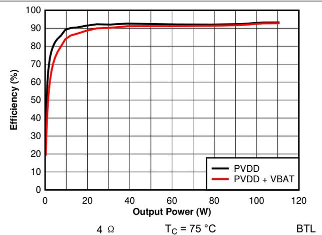
图 7-22. Efficiency vs Output Power - 4  $\Omega$  - 384 kHz
