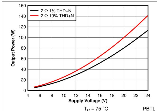
图 7-32. Output Power vs Supply Voltage - PBTL
