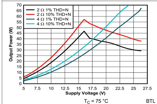
图 7-5. Output Power vs Supply Voltage
