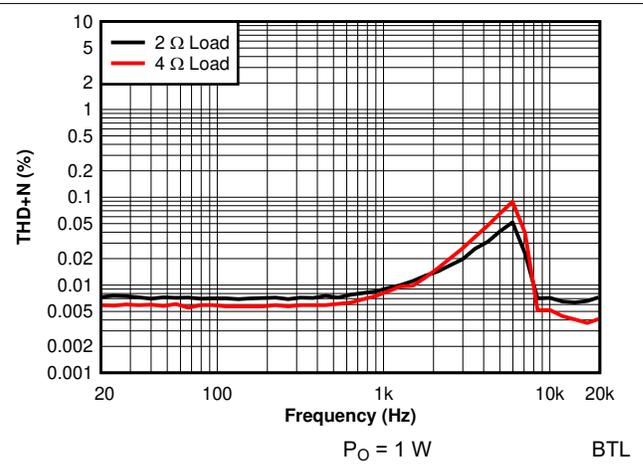
图 7-20. THD+N vs Frequency - 384 kHz
