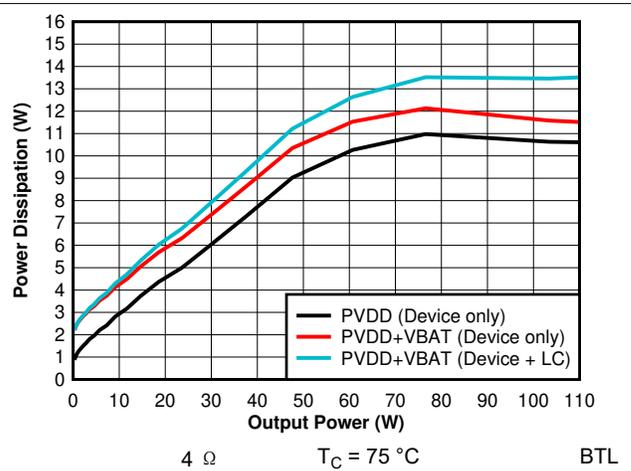
图 7-8. Power Dissipation vs Output Power - 14.4 V - 4  $\Omega$
