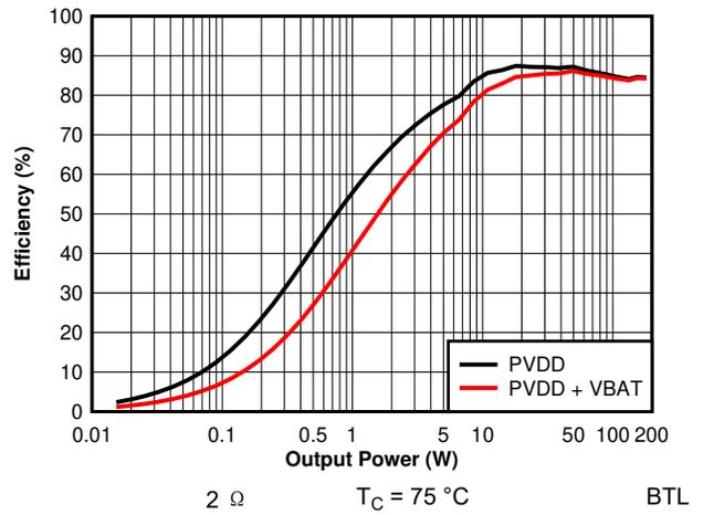
图 7-26. Efficiency vs Output Power - 2  $\Omega$  - 384 kHz (Zoomed)
