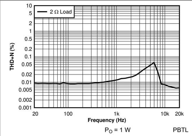
图 7-38. THD+N vs Frequency - PBTL - 384 kHz
