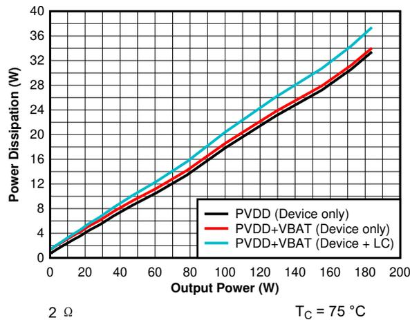
图 7-27. Power Dissipation vs Output Power - 2  $\Omega$  - 384 kHz
