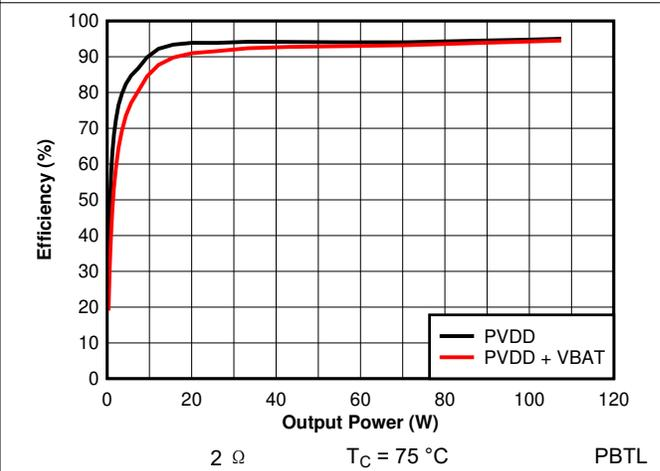
图 7-40. Efficiency vs Output Power - PBTL - 2 Ohm - 384 kHz
