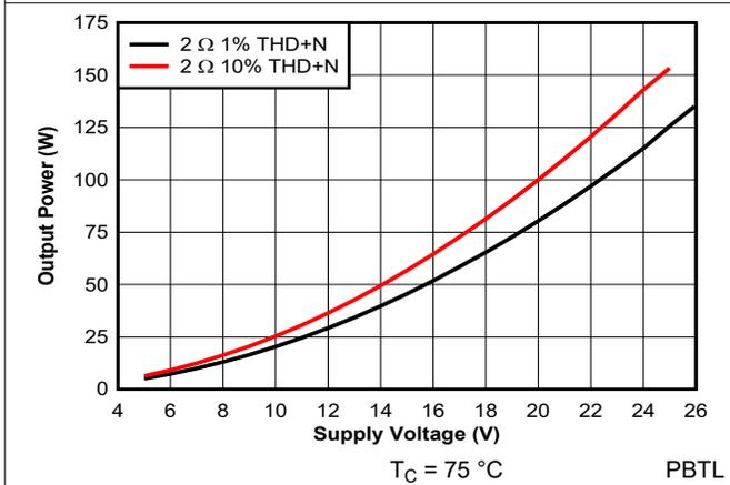
图 7-39. Output Power vs Supply Voltage - PBTL - 384 kHz
