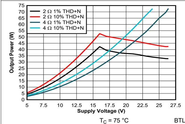
图 7-21. Output Power vs Supply Voltage - 384 kHz
