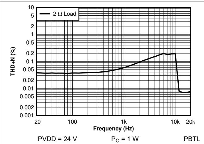
图 7-31. THD+N vs Frequency - PBTL - 24 V
