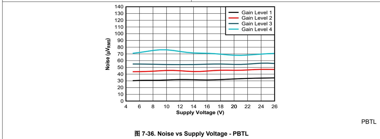
图 7-36. Noise vs Supply Voltage - PBTL
