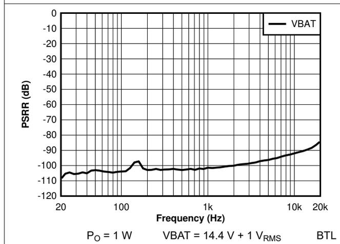
图 7-17. PSRR vs Frequency - VBAT Only
