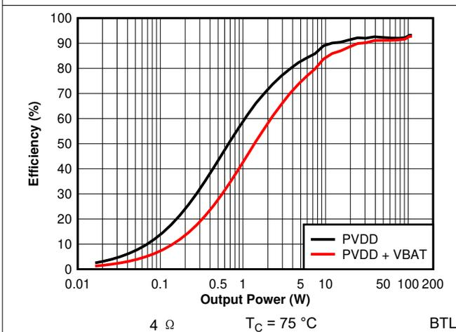
图 7-23. Efficiency vs Output Power - 4  $\Omega$  - 384 kHz (Zoomed)
