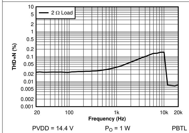
图 7-30. THD+N vs Frequency - PBTL - 14.4 V
