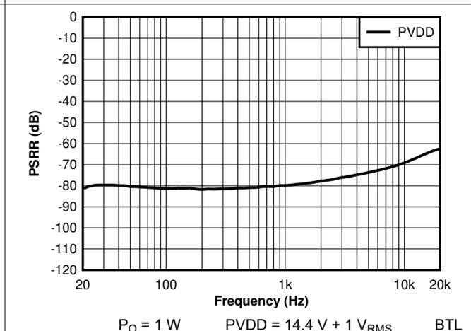
图 7-16. PSRR vs Frequency - PVDD Only
