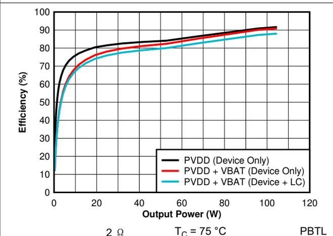
图 7-33. Efficiency vs Output Power - PBTL - 2  $\Omega$
