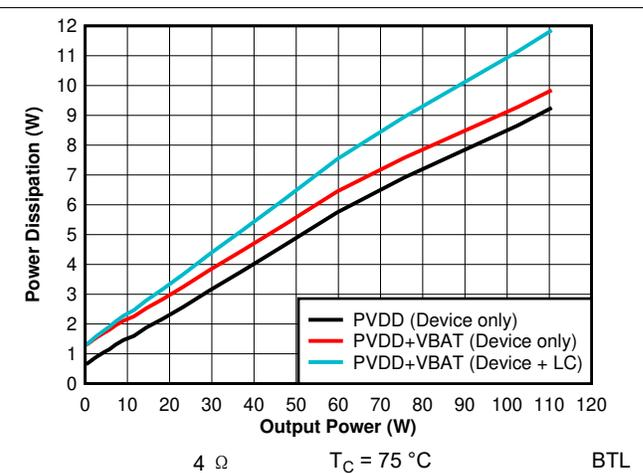
图 7-24. Power Dissipation vs Output Power - 4  $\Omega$  - 384 kHz
