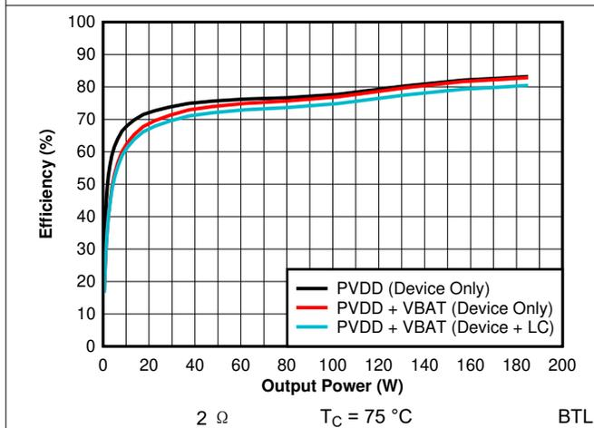
图 7-9. Efficiency vs Output Power - 14.4 V - 2  $\Omega$
