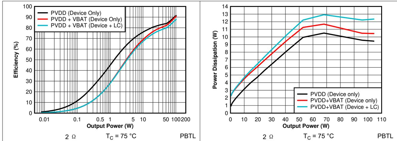
图 7-34. Efficiency vs Output power - PBTL - 2  $\Omega$  (Zoomed)
