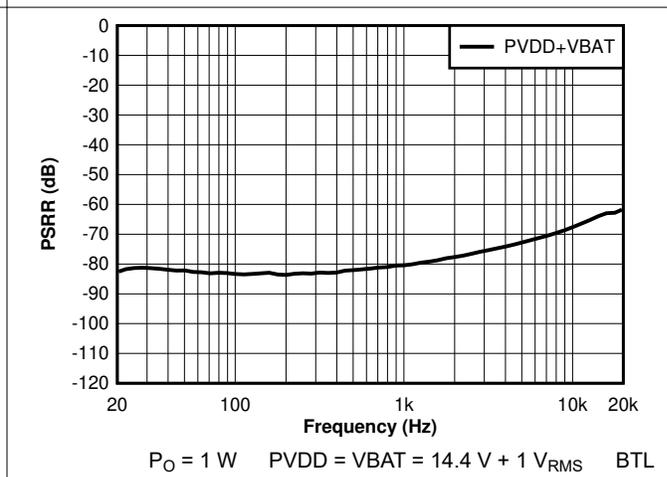
图 7-18. PSRR vs Frequency - PVDD + VBAT
