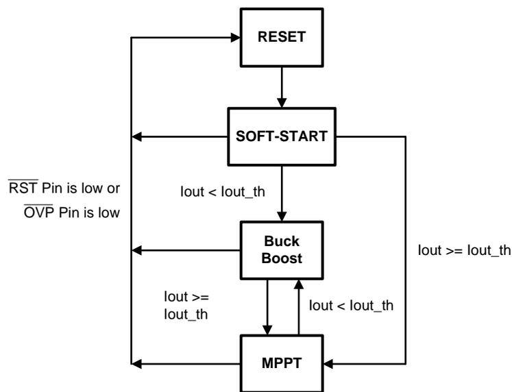
**Figure 4. High Level State Diagram for Startup**
