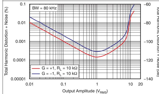
Figure 17. THD+N vs Output Amplitude
