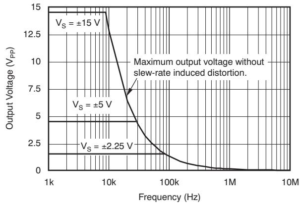
Figure 36. Maximum Output Voltage vs Frequency
