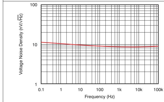
Figure 15. Input Voltage Noise Spectral Density vs Frequency
