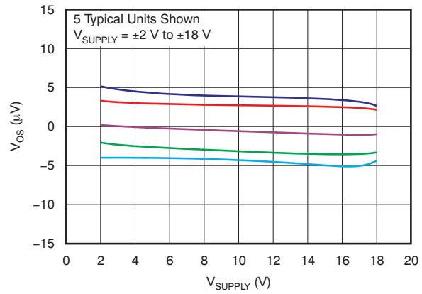
Figure 6. Offset Voltage vs Power Supply
