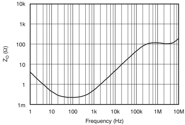
Figure 23. Open-Loop Output Impedance vs Frequency
