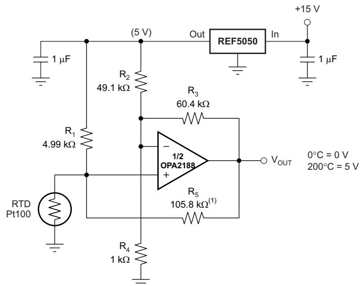
(1)  $R_5$  provides positive-varying excitation to linearize output.
