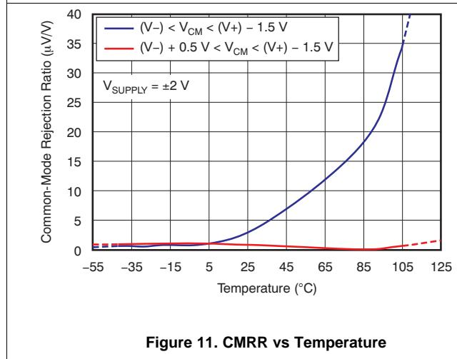
Figure 11. CMRR vs Temperature
