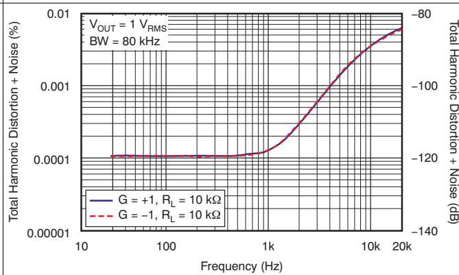
Figure 16. THD+N Ratio vs Frequency
