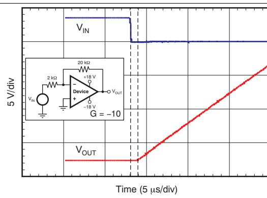
**Figure 28. Negative Overload Recovery**
