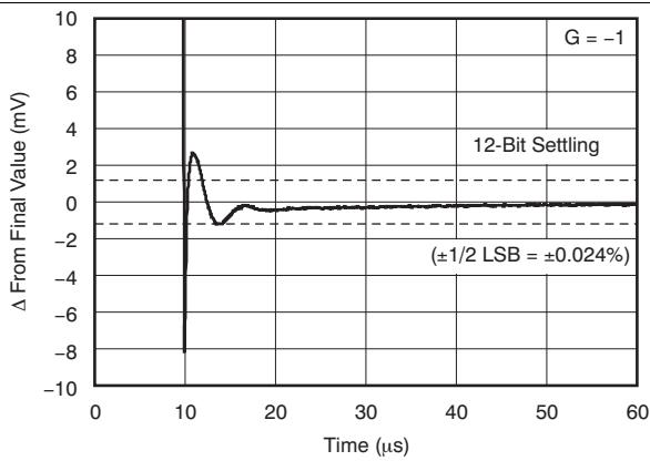
Figure 34. Large-Signal Settling Time (10-V Negative Step)
