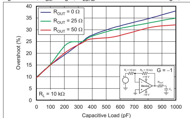
**Figure 25. Small-Signal Overshoot vs Capacitive Load (100-mV Output Step)**
