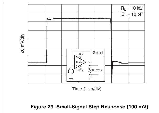
**Figure 29. Small-Signal Step Response (100 mV)**
