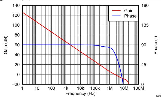
Figure 20. Open-Loop Gain and Phase vs Frequency
