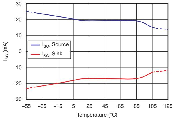
Figure 35. Short-Circuit Current vs Temperature
