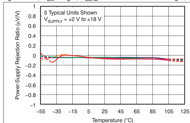
Figure 13. PSRR vs Temperature
