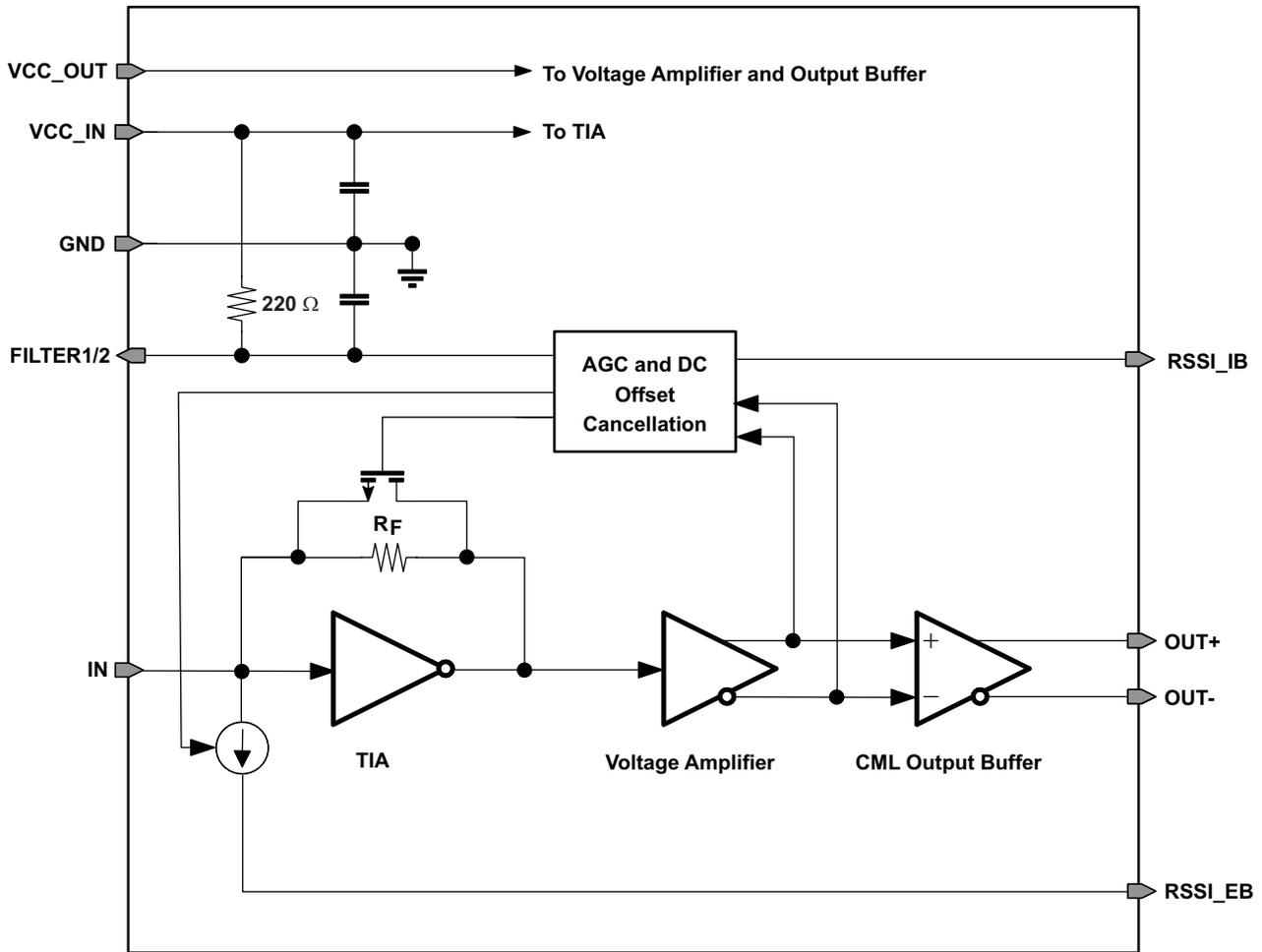
Figure 1. Simplified Block Diagram of the ONET8541T
