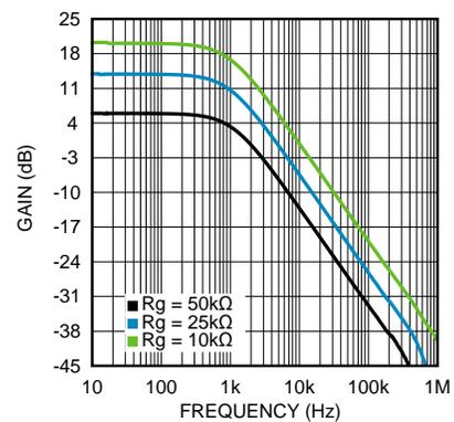
Figure 6. Gain vs. Frequency (BW = 1kHz)
