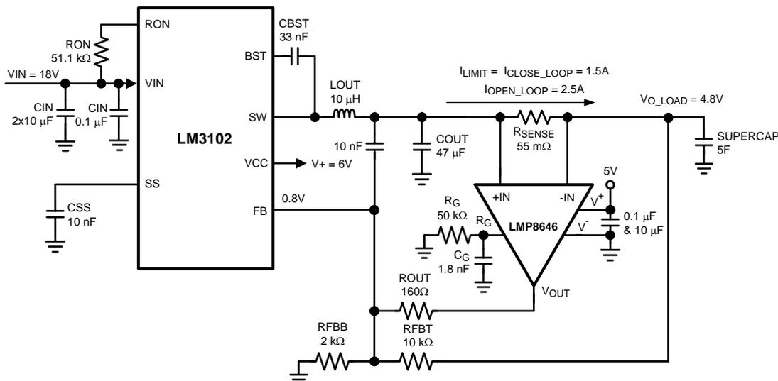
Figure 28. SuperCap Application With LM3102 Regulator
