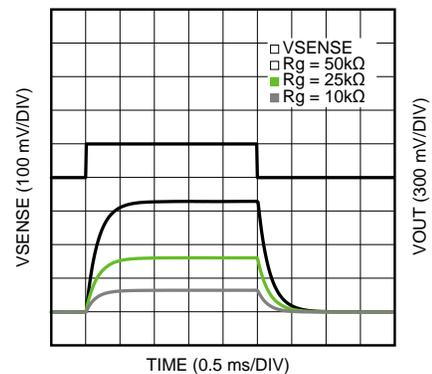
Figure 16. Large Step Response at  $\text{BW} = 1\text{ kHz}$
