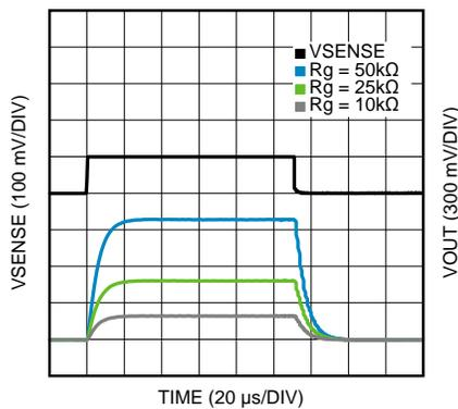
Figure 17. Large Step Response at  $\text{BW} = 35\text{ kHz}$
