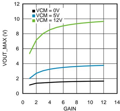
Figure 13.  $V_{\text{OUT\_MAX}}$  vs. Gain at  $V_S = 12\text{ V}$
