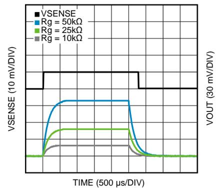
Figure 18. Small Step Response at  $\text{BW} = 1\text{ kHz}$
