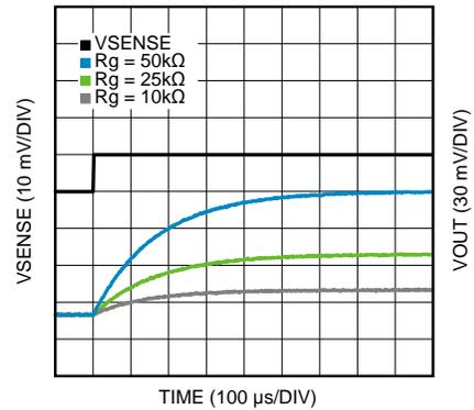
Figure 20. Settling Time (Rise) at 1 kHz
