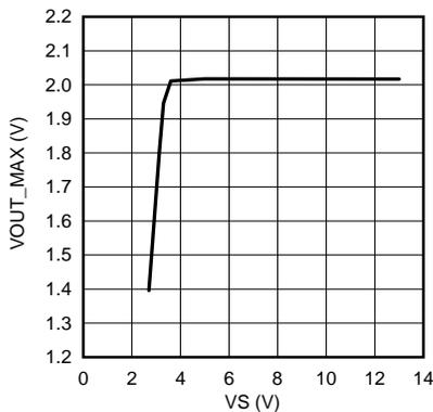
Figure 15.  $V_{\text{OUT\_MAX}}$  vs.  $V_S$  at  $V_{\text{CM}} = 2.1\text{ V}$
