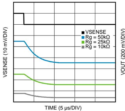
Figure 23. Settling Time (Fall) at 35 kHz
