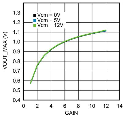
Figure 11.  $V_{\text{OUT\_MAX}}$  vs. Gain at  $V_S = 2.7\text{ V}$
