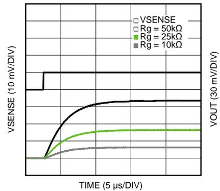
Figure 22. Settling Time (Rise) at 35 kHz
