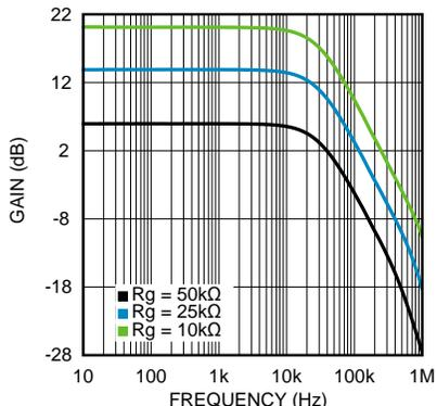
Figure 7. Gain vs. Frequency (BW = 35 kHz)
