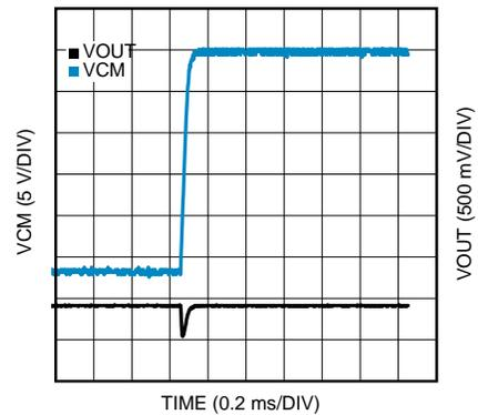
Figure 24. Common-Mode Step Response (Rise) at 35 kHz
