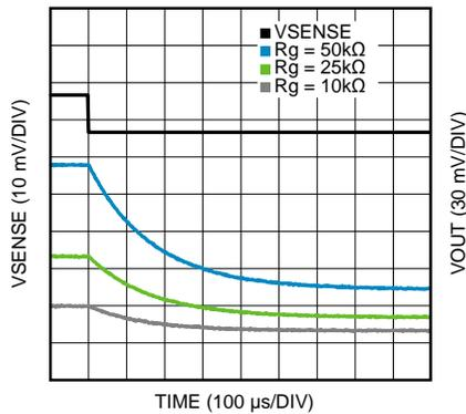
Figure 21. Settling Time (Fall) at 1 kHz
