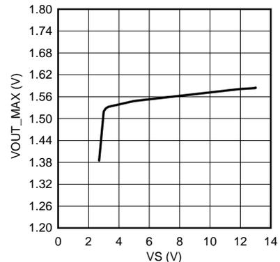
Figure 14.  $V_{\text{OUT\_MAX}}$  vs.  $V_S$  at  $V_{\text{CM}} = -2\text{ V}$
