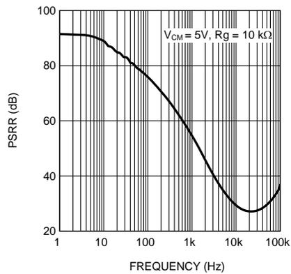
Figure 3. AC PSRR vs. Frequency
