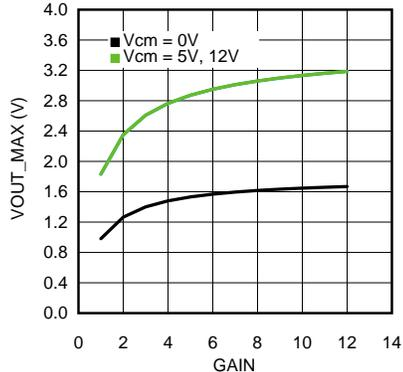
Figure 12.  $V_{\text{OUT\_MAX}}$  vs. Gain at  $V_S = 5.0\text{ V}$
