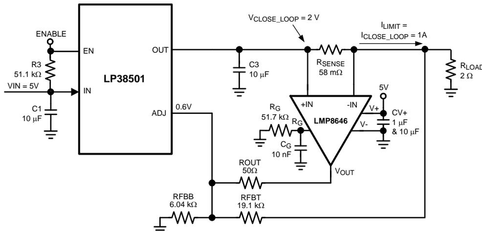
Figure 32. Resistive Load Application With LP38501 Regulator
