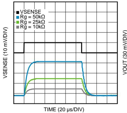
Figure 19. Small Step Response at BW = 35 kHz
