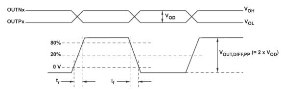
图 8-4. Output Voltage and Rise/Fall Time
