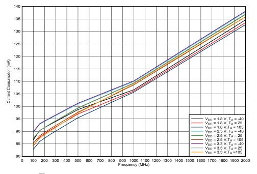
图 7-1. LMK1D2104 Current Consumption vs. Frequency
