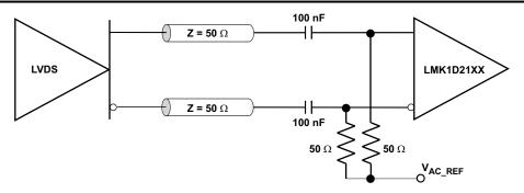
图 9-4. LVDS Clock Driver Connected to LMK1D210x Input (AC-Coupled)
