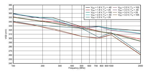
图 7-2. LMK1D2104 VOD vs. Frequency
