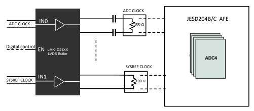
图 10-1. Fan-Out Buffer for ADC Device clock and SYSREF distribution
