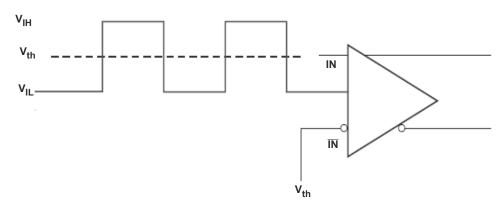
图 8-3. DC-Coupled LVCMOS Input During Device Test
