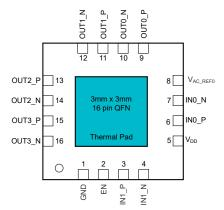
图 6-1. LMK1D2102: RGT Package 16-Pin VQFN Top View
