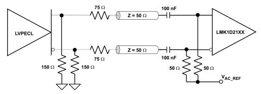
图 9-5. LVPECL Clock Driver Connected to LMK1D210x Input
