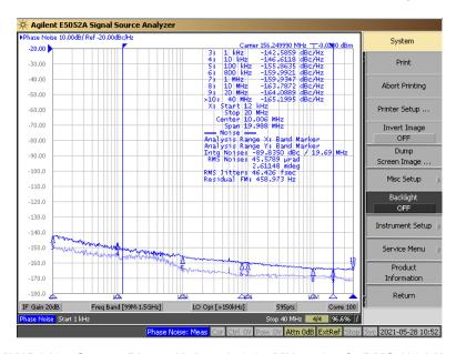
图 10-4. LMK1D2104 Output Phase Noise, 156.25 MHz, 46.4-fs RMS (12 kHz to 20 MHz)
