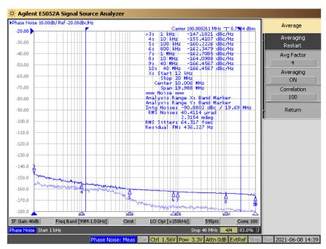
图 10-5. LMK1D2104 Output Phase Noise, 100 MHz, 1 kHz offset: -147 dBc/Hz
