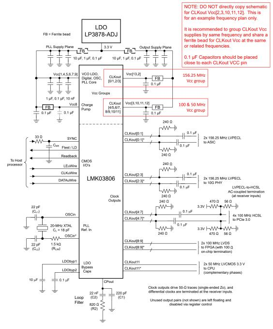
图 8-13. Example Network Line Card Application
