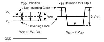
图 6-2. Two Different Definitions for Differential Output Signals
