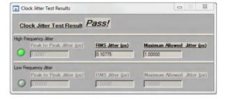
图 8-12. PCIe 3.0 RMS Jitter, 100-MHz HCSL
