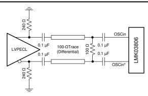
图 8-5. OSCin/OSCin\* Termination for an LVPECL Reference Clock Source
