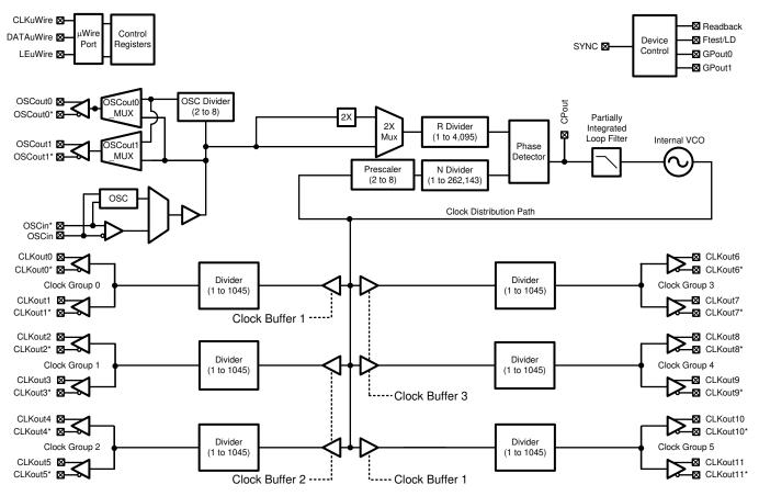
图 7-1. Detailed LMK03806 Block Diagram
