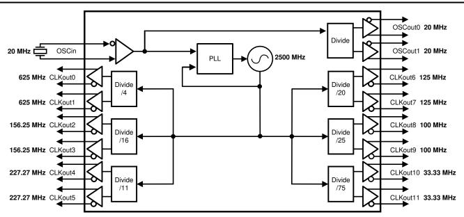
图 7-2. 10-Gigabit Ethernet Reference Clocks
