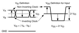
图 6-1. Two Different Definitions for Differential Input Signals
