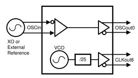
图 7-5. Start-Up Clock Using Crystal Reference
