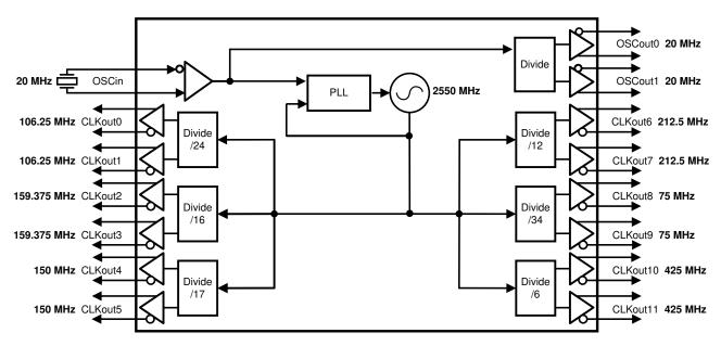
图 7-3. Fiber Channel Reference Clocks
