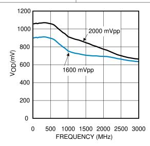
图 5-4. LVPECL With 120- $\Omega$  Emitter Resistors V<sub>OD</sub> vs Frequency
