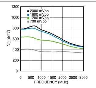
图 5-3. LVPECL With 240-Ω Emitter Resistors V<sub>OD</sub> vs Frequency
