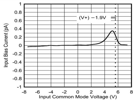
图 5-4. Input Bias Current vs Input Common-Mode Voltage
