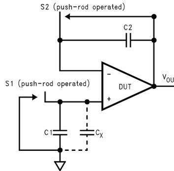
图 6-5. Simple Input Bias Current Test Circuit
