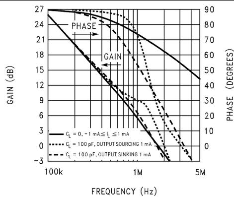
图 5-11. Frequency Response vs Capacitive Load
