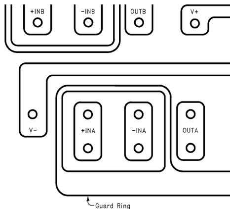
**图 6-16. Example of Guard Ring in PCB Layout**
