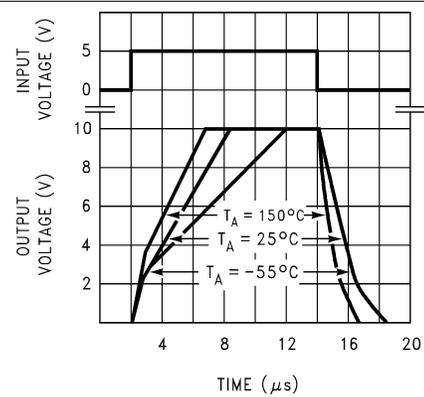
图 5-12. Noninverting Large-Signal Pulse Response
