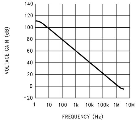
图 5-10. Open-Loop Frequency Response
