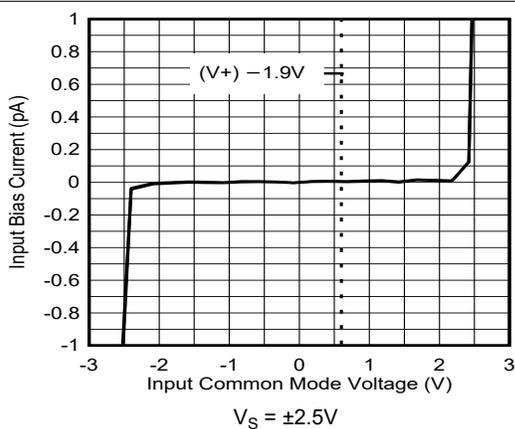
图 5-5. Input Bias Current vs Input Common-Mode Voltage
