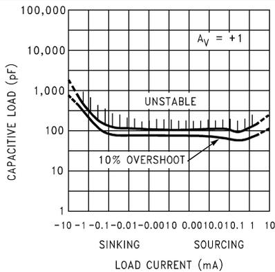
图 5-15. Stability vs Capacitive Load
