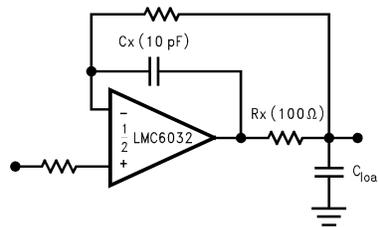
**图 6-3. Rx, Cx Improve Capacitive Load Tolerance**
