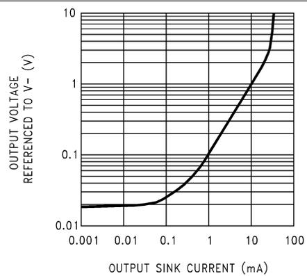
图 5-6. Output Characteristics Current Sinking
