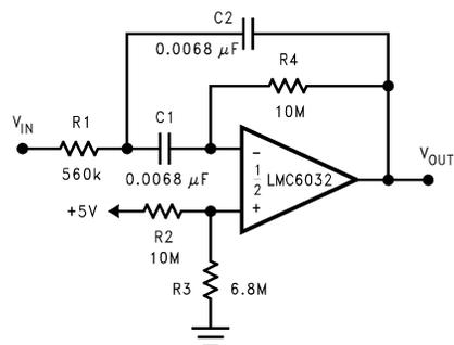
$$f_0 = 10\text{Hz}, Q = 2.1, \text{gain} = -8.8$$
