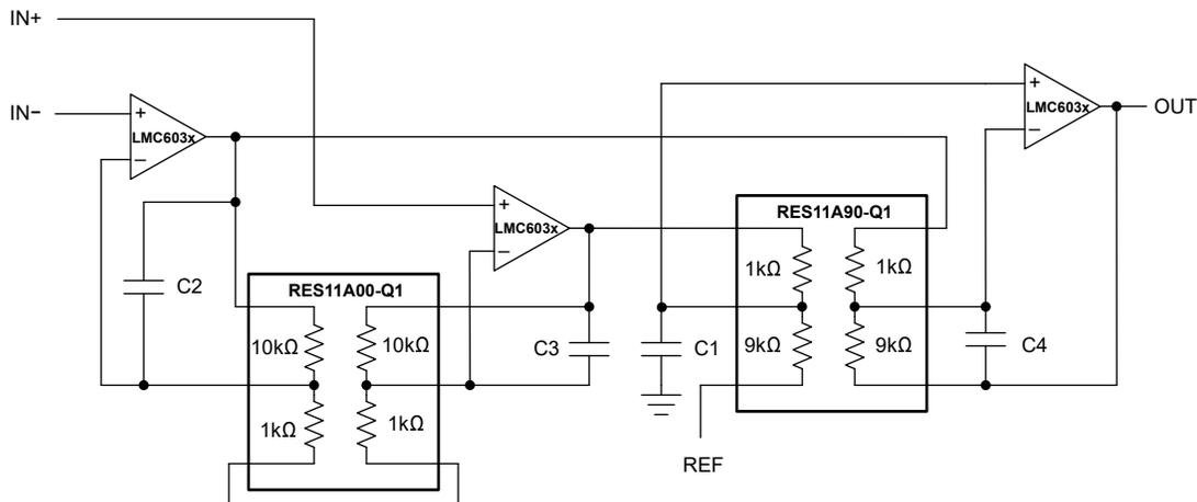
图 6-7. Improved Instrumentation Amplifier With RES11A
