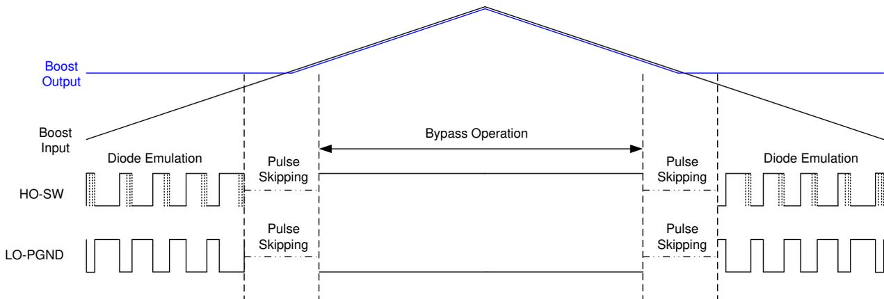
图 8-18. PWM to Bypass Transition in DCM Operation
