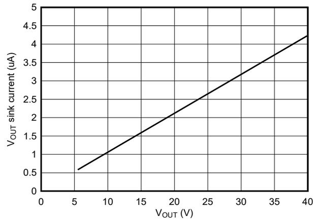
图 7-14.  $V_{OUT}$  Sink Current vs  $V_{OUT}$  (Deep Sleep)
