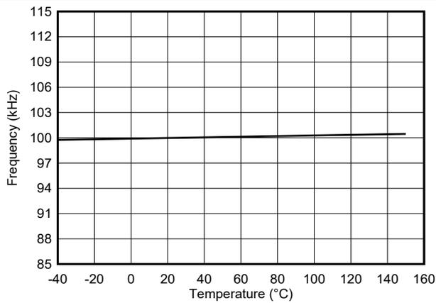
图 7-3. Frequency vs Temperature
