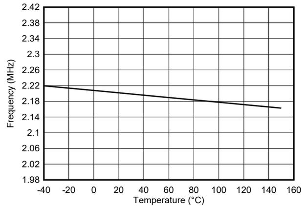
图 7-2. Frequency vs Temperature
