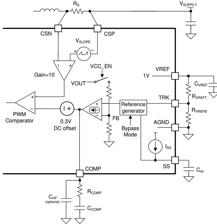
图 8-13. Error Amplifier, Current Sense Amplifier, and PWM
