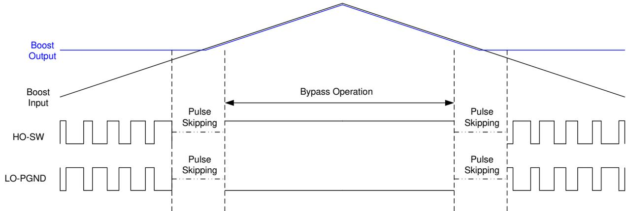
图 8-17. PWM to Bypass Transition in CCM Operation
