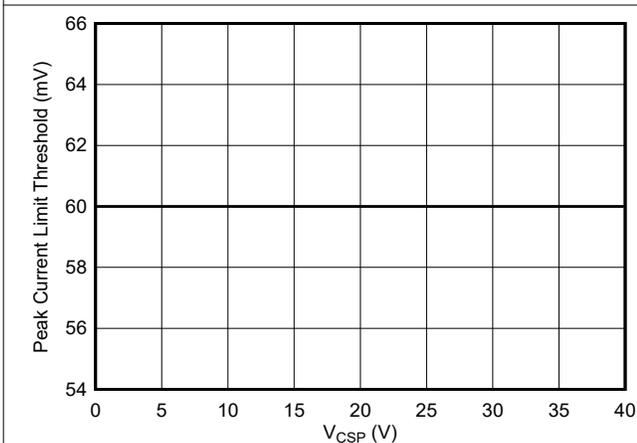
图 7-11. Peak Current Limit Threshold vs  $V_{CSP}$
