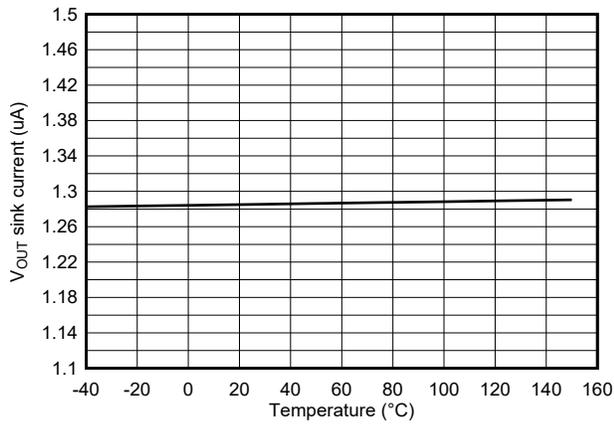
图 7-15.  $V_{OUT}$  Sink Current vs Temperature (Deep Sleep)
