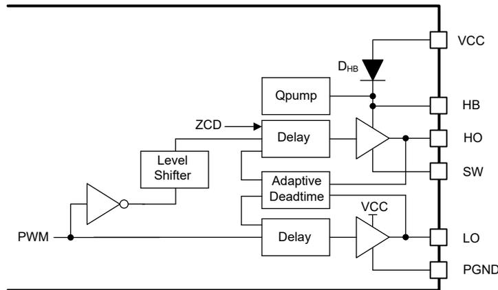
图 8-19. Driver Structure with Internal Boot Diode
