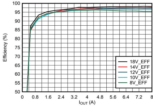
图 9-4. Efficiency vs.  $I_{OUT}$ ,  $V_{OUT} = 24\text{ V}$  (FPWM)
