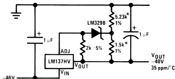
\*Use resistors with good tracking TC < 25 ppm/°C
