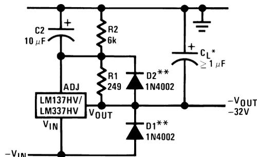
\*When  $C_L$  is larger than 20  $\mu F$ , D1 protects the LM137HV in case the input supply is shorted
