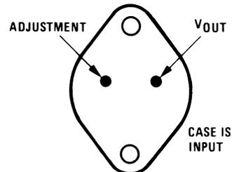
**Figure 2. TO-3 Package (Bottom View)**
