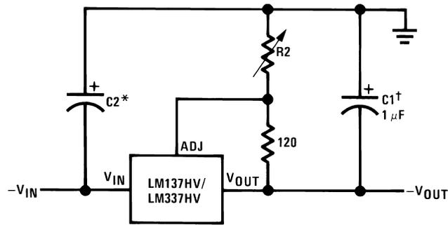
$$-V_{OUT} = -1.25V \left( 1 + \frac{R_2}{120\Omega} \right) + \left[ -I_{Adj}(R_2) \right]$$
