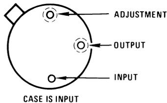
**Figure 1. TO Package – Bottom View**
