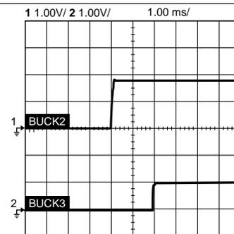
Figure 18. From Buck 2 Start-Up to Buck 3 Start-Up
