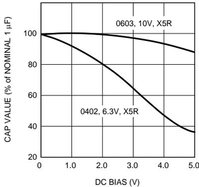
Figure 26. Typical Variation in Capacitance vs DC Bias
