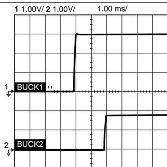
Figure 17. From Buck 1 Start-Up to Buck 2 Start-Up
