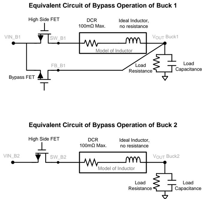
Figure 21. Bypass Operations for Buck 1 and Buck 2
