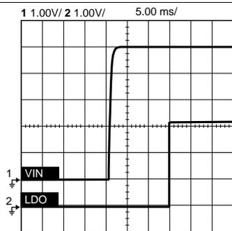
Figure 15. LDO Start-Up Time from  $V_{IN}$  Rise
