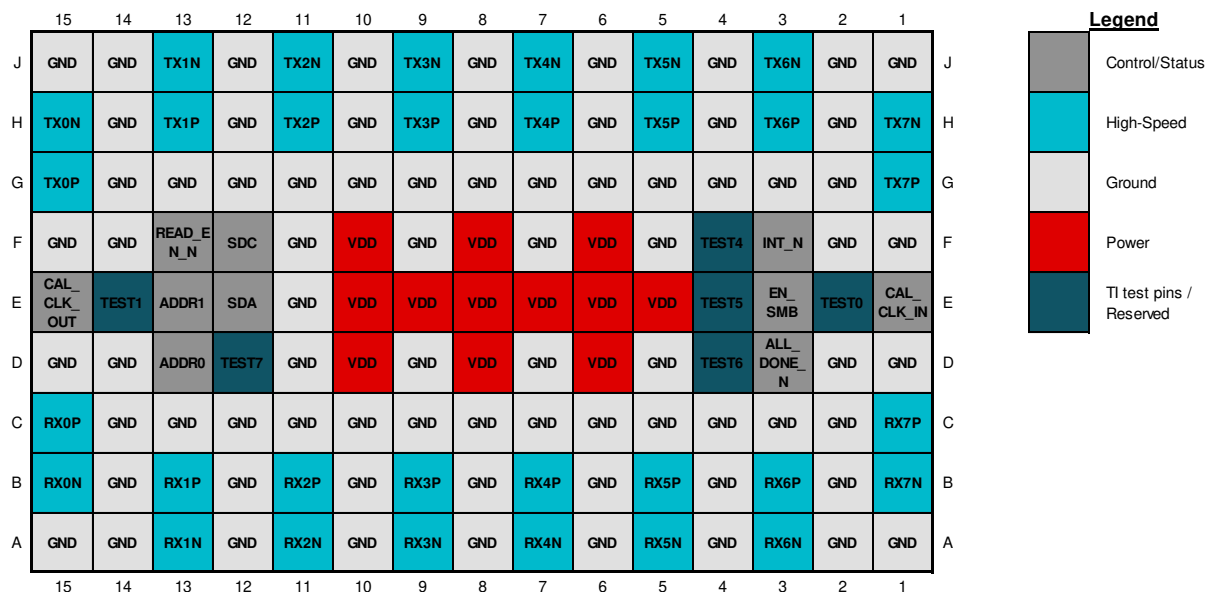
图 4-1. 135-Pin fcBGA, 0.8mm BGA Pin Pitch (Top View)
