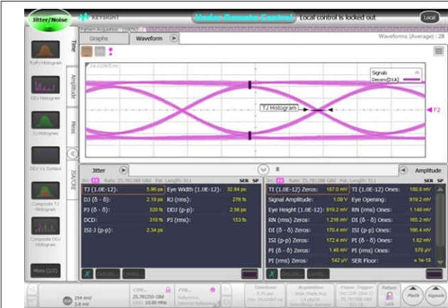
9-5 shows a typical output eye diagram for the DS250DF230 operating at 25.78125 Gbps with PRBS9 pattern using FIR main-cursor of +28, pre-cursor of 0 and post-cursor of +3. All other device settings are left at default.
