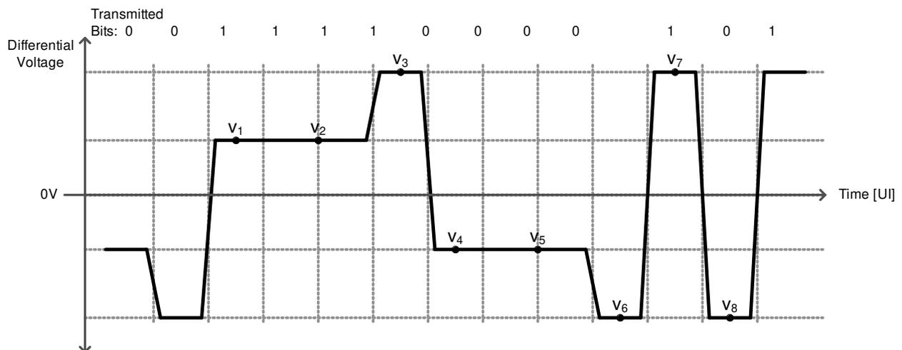
图 8-3. Conceptual FIR Waveform With Pre-Cursor Only
