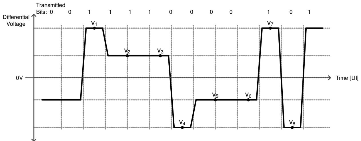
图 8-2. Conceptual FIR Waveform With Post-Cursor Only
