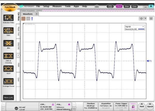
9-6 shows an example of DS250DF230 FIR transmit equalization while operating at 25.78125 Gbps. In this example, the Tx FIR filter main-cursor is set to +25, post-cursor to -3 and pre-cursor to -3. An 8T pattern is used to evaluate the FIR filter, which consists of 0xFF00. All other device settings are left at default.
