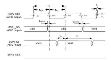
图 6-8. Synchronous Serial Port Interface—Secondary
