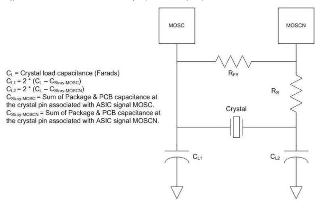
图 8-3. Recommended Crystal Oscillator Configuration
