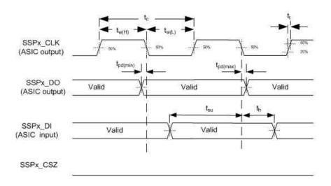
图 6-7. Synchronous Serial Port Interface—Primary
