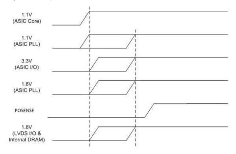
图 9-1. System Power-Up Sequence
