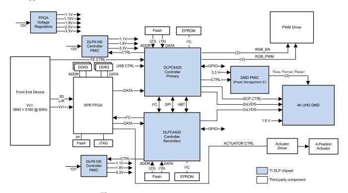
图 8-1. Typical 4K UHD LED Display Application
