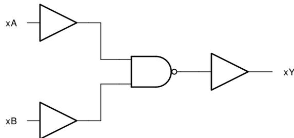
图 8-1. Logic Diagram (Positive Logic) for the CD74HC00
