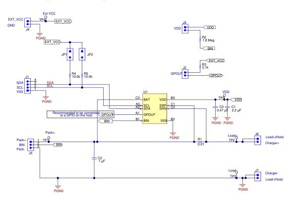
图 8-1. Typical Application with High-Side Current Sense Resistor
