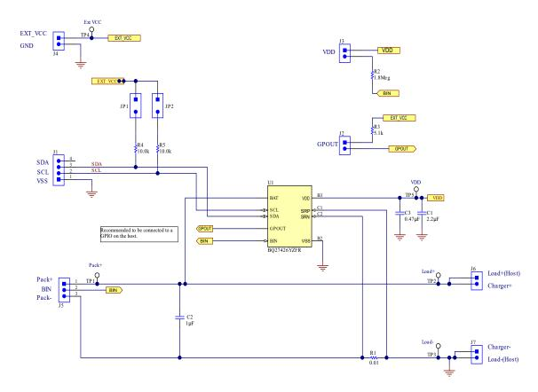
图 8-2. Typical Application with Low-Side Current Sense Resistor
