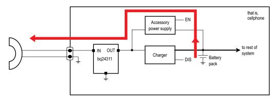
Figure 13. Powering an Accessory - The Red Arrows Show the Direction of Current Flow
