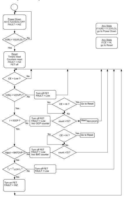
Figure 10. Flow Diagram
