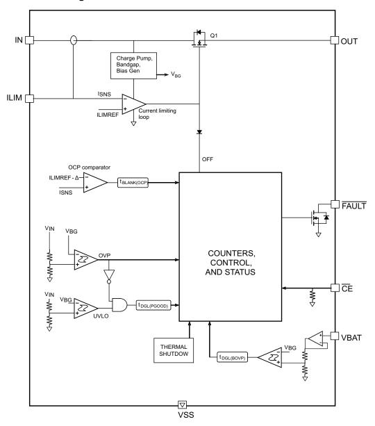
Figure 9. Simplified Block Diagram
