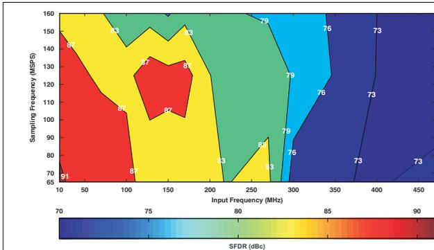
图 6-33. Spurious-Free Dynamic Range (0dB Gain)
