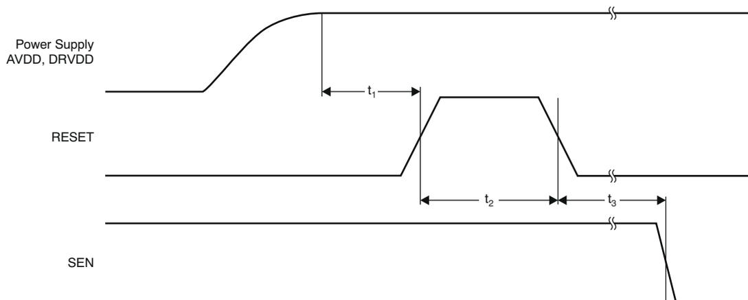
NOTE: A high pulse on the RESET terminal is required in the serial interface mode when initialized through a hardware reset. For parallel interface operation, RESET must be permanently tied high.
