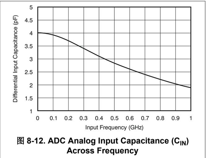
show the impedance ( $Z_{IN} = R_{IN} \parallel C_{IN}$ ) looking into the ADC input terminals.
