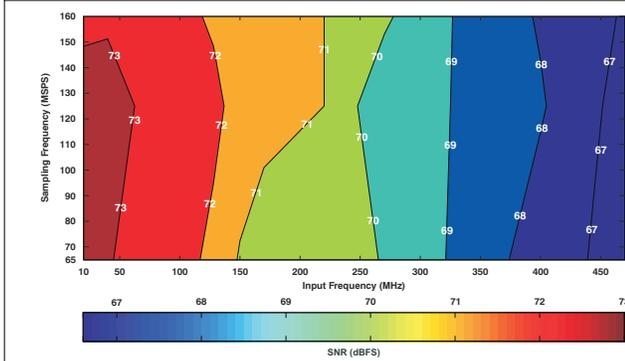
图 6-35. Signal-To-Noise Ratio (0dB Gain)
