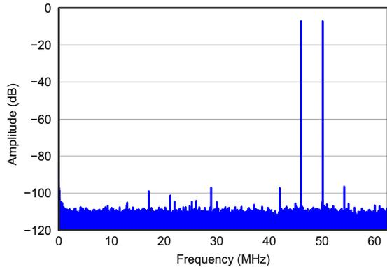
Each Tone at  $-7\text{dBFS}$  Amplitude  $f_{IN1} = 46\text{MHz}$
