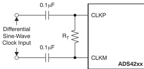
A. R<sub>T</sub> = termination resistor, if necessary.
