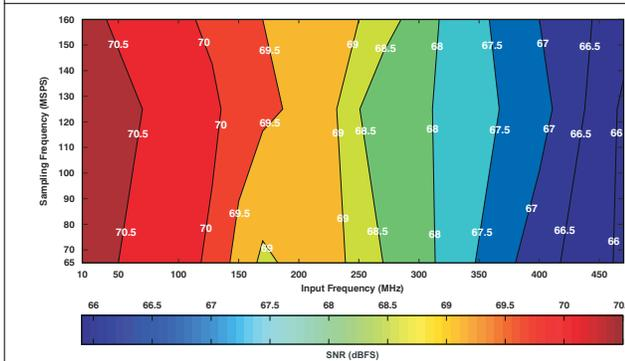
图 6-37. Signal-To-Noise Ratio (0dB Gain)
