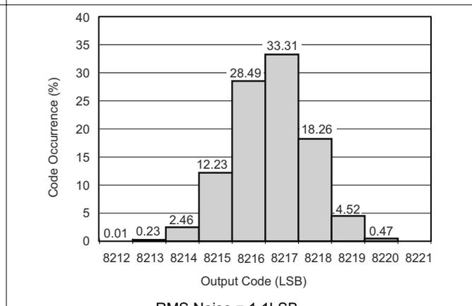
图 6-27. Output Noise Histogram (With Inputs Shorted To VCM)
