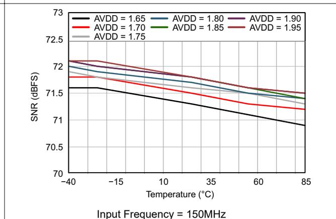
图 6-21. SNR vs Temperature And AVDD Supply
