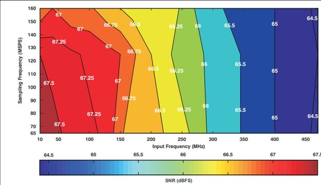
图 6-36. Signal-To-Noise Ratio (6dB Gain)
