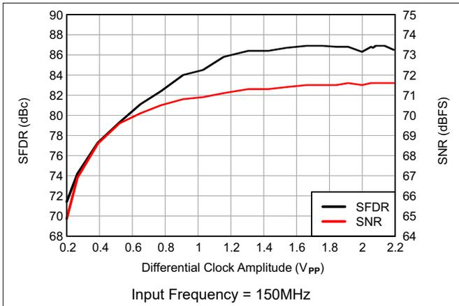
图 6-24. Performance vs Input Clock Amplitude
