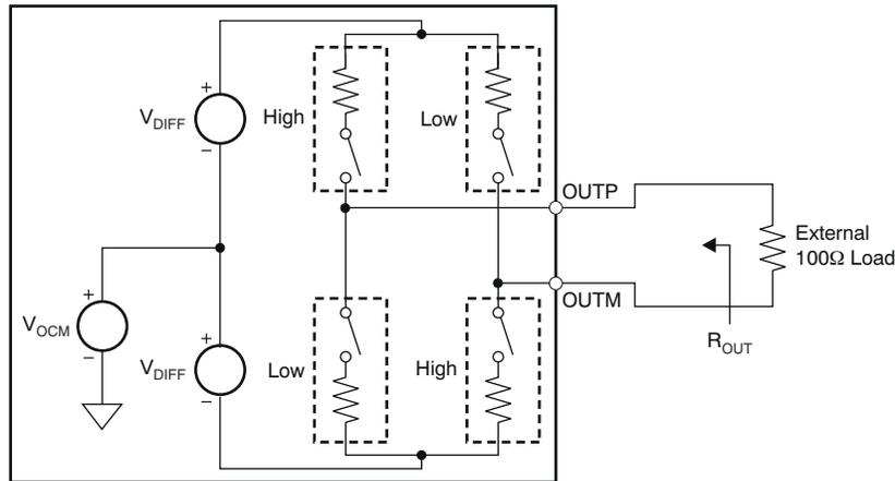
NOTE: Default swing across  $100\ \Omega$  load is  $\pm 350\text{mV}$ . Use the LVDS SWING bits to change the swing.
