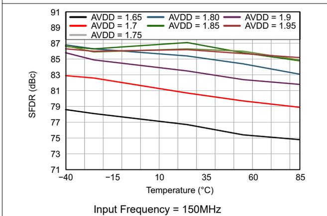
图 6-20. SFDR vs Temperature And AVDD Supply
