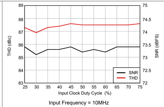
图 6-25. Performance vs Input Clock Duty Cycle
