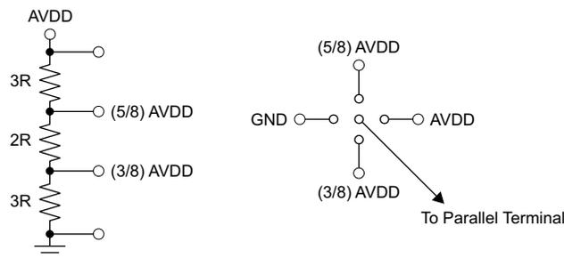
图 7-8. Simple Scheme To Configure The Parallel Terminals
