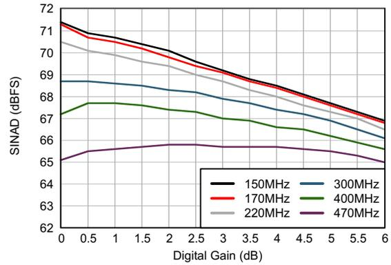
图 6-15. SINAD vs Gain And Input Frequency
