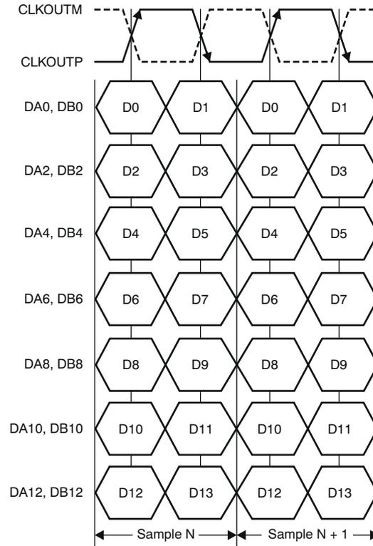
图 6-5. ADS4245 LVDS Interface Timing Diagram
