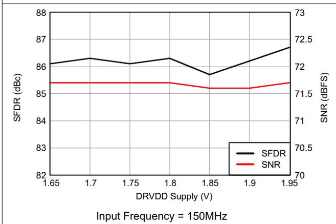
图 6-22. Performance vs DRVDD Supply Voltage
