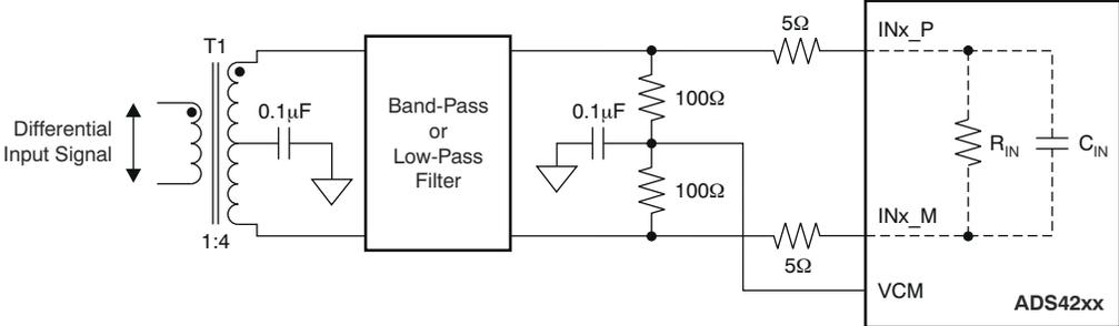
. Such filters present low source impedance at the high frequencies corresponding to the sampling glitch and help avoid the performance loss with the high source impedance.
