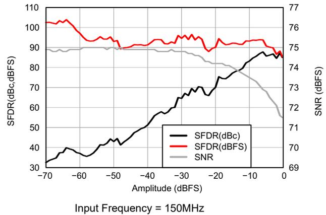
图 6-17. Performance vs Input Amplitude
