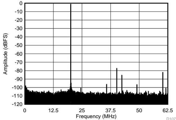
图 7. FFT for 270-MHz Input Signal (Dither On)
