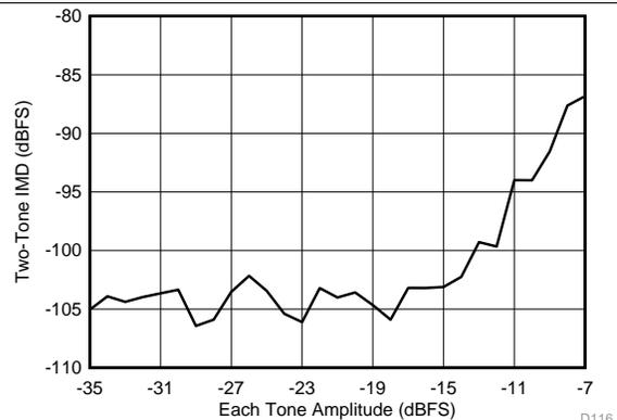
$f_{IN1} = 185 \text{ MHz}$ ,  $f_{IN2} = 190 \text{ MHz}$
