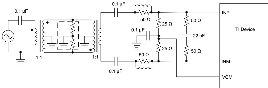
图 85. Driving Circuit for Low Input Frequencies
