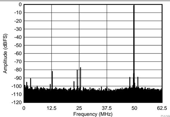
图 9. FFT for 450-MHz Input Signal (Dither On)
