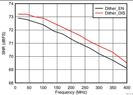
图 17. Signal-to-Noise Ratio vs Input Frequency
