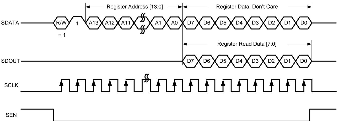
图 55. Serial Register Read Timing Diagram
