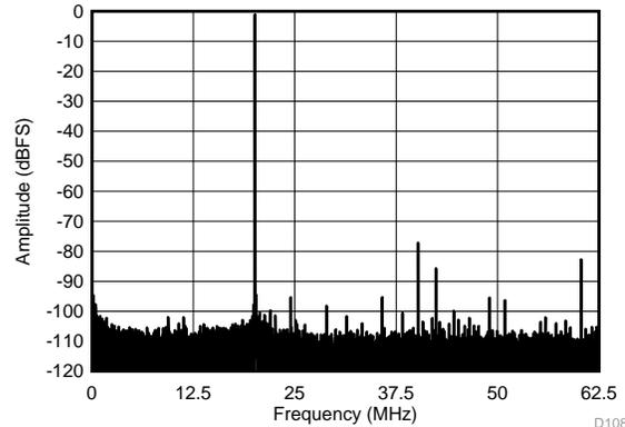
图 8. FFT for 270-MHz Input Signal (Dither Off)
