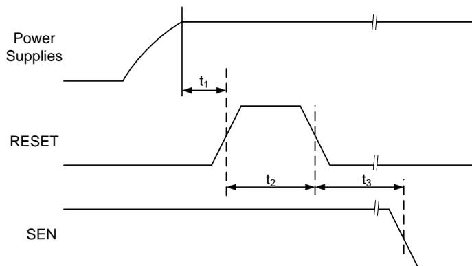
图 57. Initialization of Serial Registers after Power-Up
