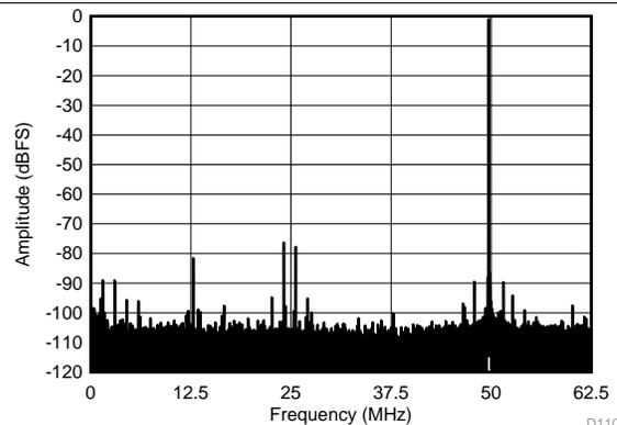
图 10. FFT for 450-MHz Input Signal (Dither Off)
