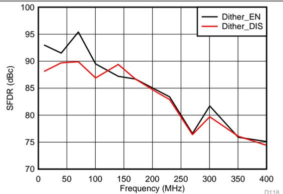
图 18. Spurious-Free Dynamic Range vs Input Frequency
