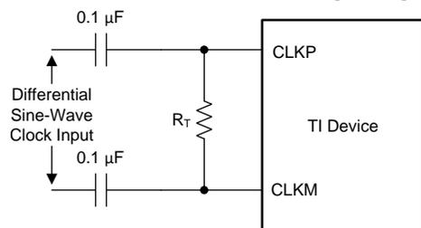
NOTE:  $R_T$  = termination resistor, if necessary.
