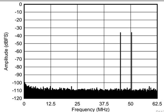
图 12. FFT for Two-Tone Input Signal
