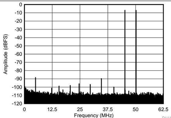
图 11. FFT for Two-Tone Input Signal
