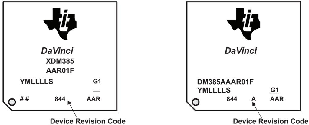
Figure 1. Example, Device Revision Codes (AAR Package)
