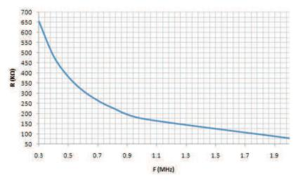
Figure 15. ROSC vs Switching Frequency
