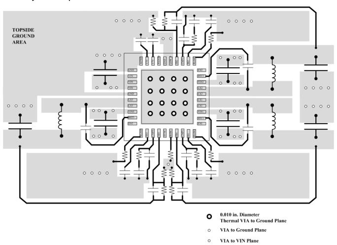
Figure 35. Layout Schematic
