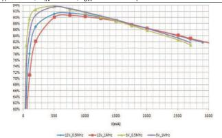
$V_{OUT}$  = 2.5 V, L = 4.7  $\mu$ H, DCR = 28  $m\Omega$  (Also Applies to Buck 2)
