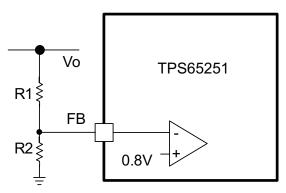
Figure 16. Voltage Divider Circuit
