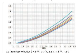
Figure 36. Buck 1 Losses (W) vs Output Current  $V_{\rm IN}$  = 12 V,  $f_{\rm SW}$  = 500 kHz
