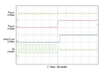
t - Time - 20 ms/div Figure 8. Full-Load to Short-Circuit Transient Response
