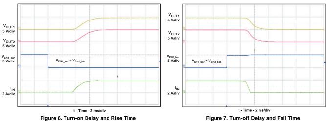
Figure 6. Turn-on Delay and Rise Time
