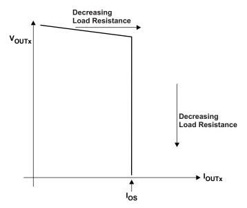
Figure 4. Output Voltage vs. Current-Limit Threshold
