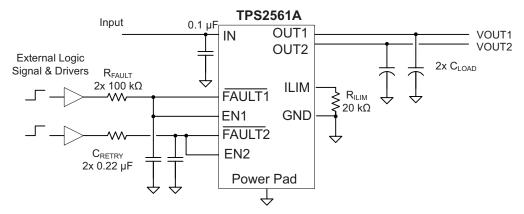
Figure 20. Auto-Retry Functionality With External EN Signal
