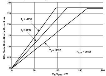
Figure 17. Switch Current vs. Drain-Source Voltage Across Switch
