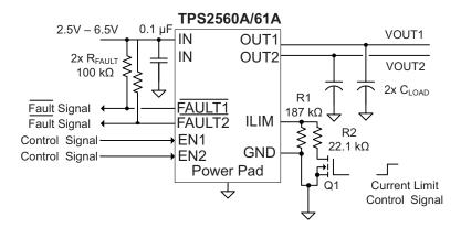
Figure 21. Two-Level Current-Limit Circuit
