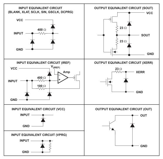
Figure 9. Input and Output Equivalent Circuits
