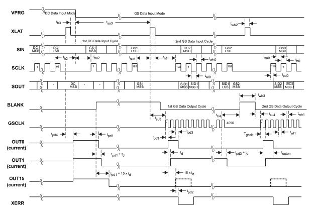
Figure 12. Serial Data Input Timing Chart
