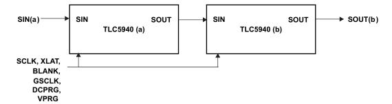
Figure 13. Cascading Two TLC5940-EP Devices
