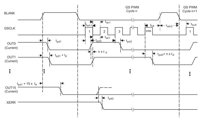
Figure 22. Grayscale PWM Cycle Timing Chart
