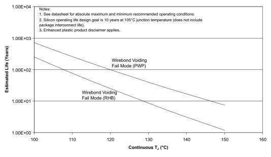
Figure 11. TLC5940-EP Mold Compound Operating Life
