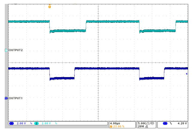
Figure 24. Output Waveform with Different Grayscale PWM Data
