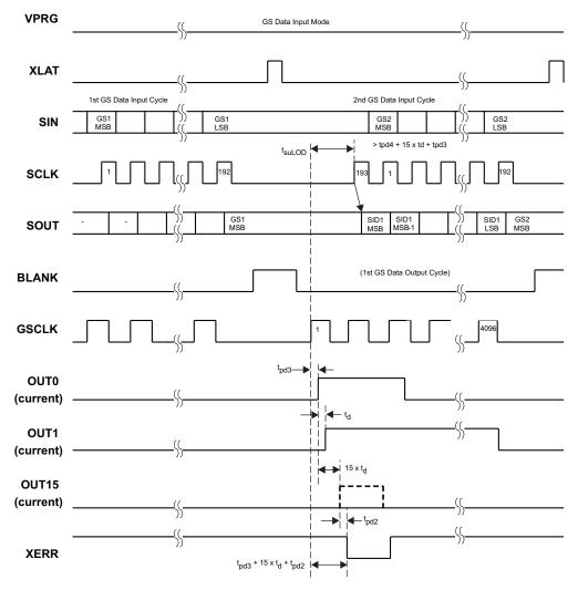
Figure 21. Readout Status Information Data (SID) Timing Chart
