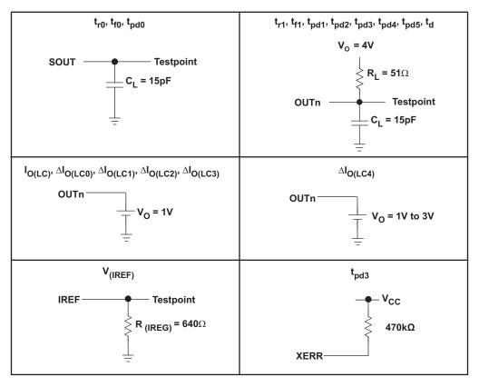
Figure 10. Parameter Measurement Circuits
