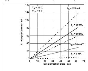
Figure 7. Output Current vs DOT Correction Linearity (ABS Value)
