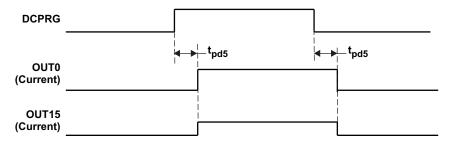
Figure 18. DCPRG and OUTn Timing Diagram
