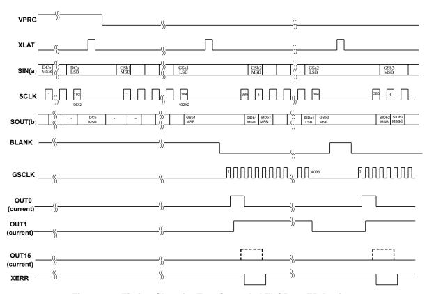
Figure 14. Timing Chart for Two Cascaded TLC5940-EP Devices
