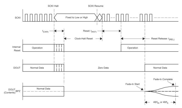
Figure 3. Clock-Halt Power-Down and Reset Timing
