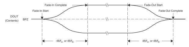
Figure 25. Fade-In and Fade-Out Operations
