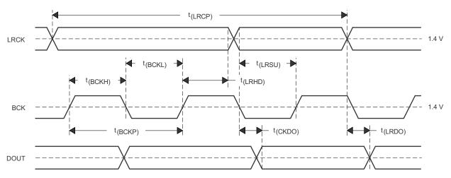
Figure 4. Audio Data Interface Timing (Slave Mode: LRCK and BCK Work as Inputs)
