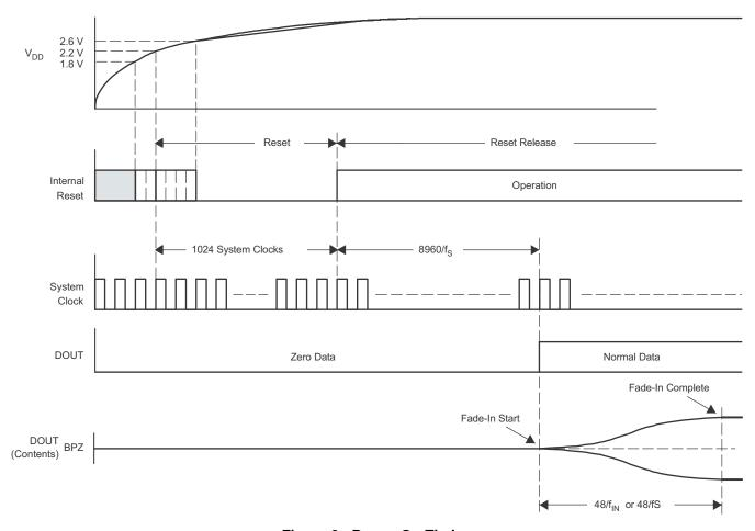
Figure 2. Power-On Timing
