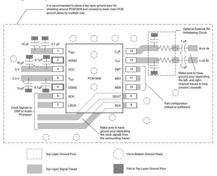
Figure 28. PCM1808 Layout Example
