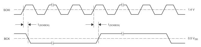
Figure 6. Audio Clock Interface Timing (Master Mode: BCK Works as Output)
