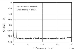
Figure 19. Output Spectrum (-0.5 dB, N = 8192)
