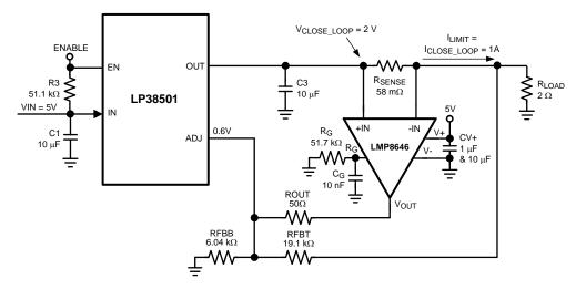
Figure 32. Resistive Load Application With LP38501 Regulator
