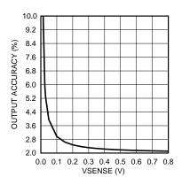
Figure 27. Output Accuracy vs. V<sub>SENSE</sub>
