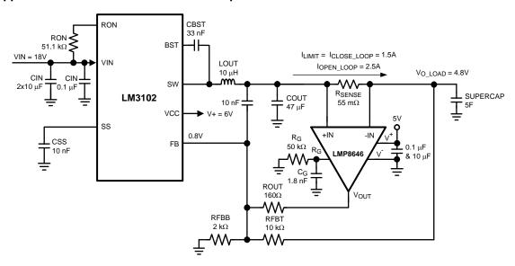
Figure 28. SuperCap Application With LM3102 Regulator
