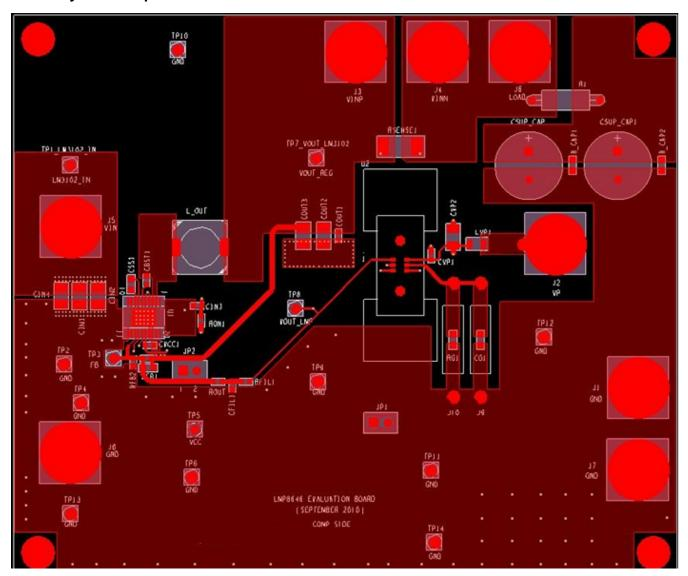
Figure 34. LMP8646 Evaluation Board Layout
