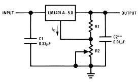
$$\begin{split} &V_{OUT}=5V+(5V/R1+I_O)~R2\\ &5V/R1=3~I_O~load~regulation~(L,)~[(R1+R2)/R1]~(L,~of~LM140LA-5.0) \end{split}$$
