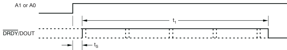
图 8-7. Example of Settling Time After Changing the Input Multiplexer
