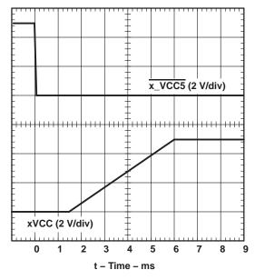
Figure 12. xVCC Propagation Delay and Rise Time With 150-μF Load, 5-V Switch
