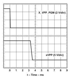
Figure 15. xVPP Propagation Delay and Fall Time With 1-μF Load, 12-V Switch
