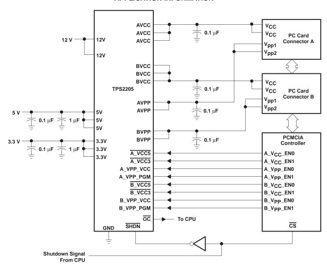
Figure 32. Detailed Interconnections and Capacitor Recommendations
