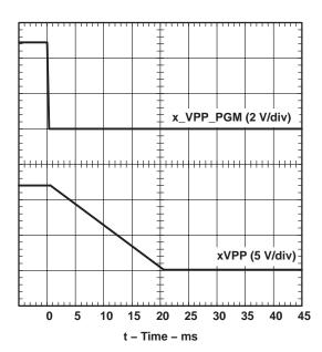
Figure 17. xVPP Propagation Delay and Fall Time With 150-μF Load, 12-V Switch
