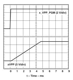
Figure 16. xVPP Propagation Delay and Rise Time With 150-μF Load, 12-V Switch
