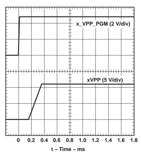
Figure 14. xVPP Propagation Delay and Rise Time With 1-μF Load, 12-V Switch
