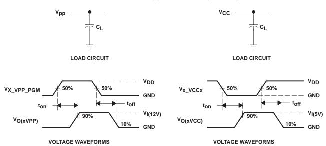
Figure 1. Test Circuits and Voltage Waveforms
