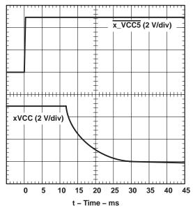
Figure 13. xVCC Propagation Delay and Fall Time With 150-μF Load, 5-V Switch
