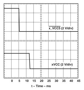
Figure 7. xVCC Propagation Delay and Fall Time With 1-µF Load, 3.3-V Switch,  $V_{I(5V)} = 0$
