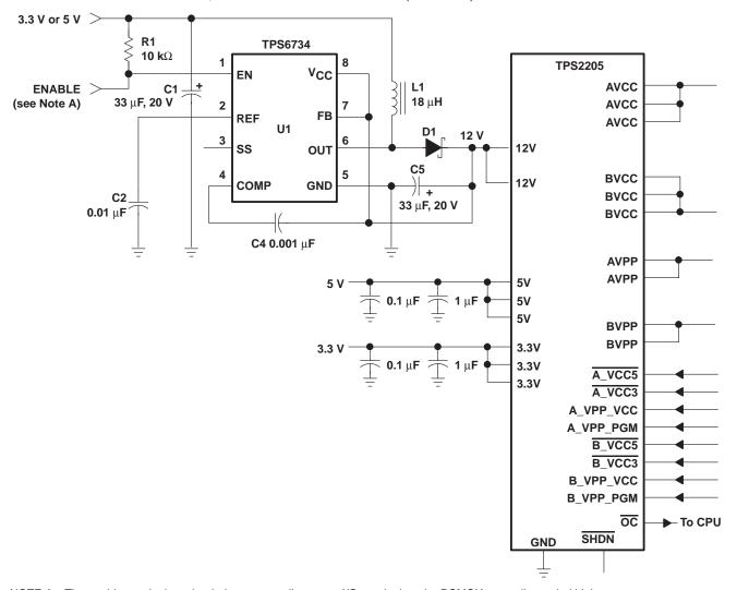
NOTE A: The enable terminal can be tied to a generall purpose I/O terminal on the PCMCIA controller or tied high.
