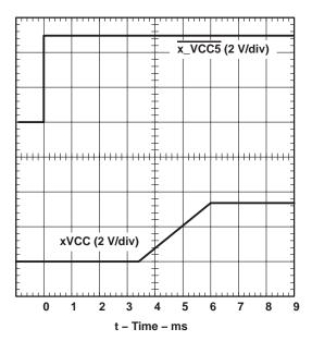
Figure 2. xVCC Propagation Delay and Rise Time With 1- $\mu$ F Load, 3.3-V Switch, (V<sub>I(5V)</sub> = 5 V)
