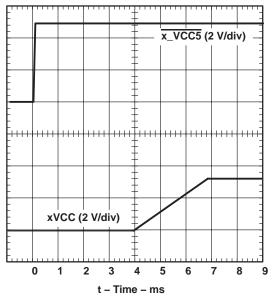
Figure 8. xVCC Propagation Delay and Rise Time With 150-µF Load, 3.3-V Switch,  $V_{I(5V)} = 0$
