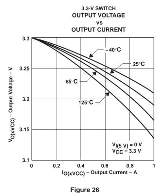
3.3-V SWITCH **OUTPUT VOLTAGE OUTPUT CURRENT** 3.3 40°C 3.27 25°C Vo(xVCC) - Output Voltage - V 85°C 3.24 125°C 3.21 3.18  $V_{I(5V)} = 5 V$ V<sub>I(3.3V)</sub> = 3.3 V V<sub>CC</sub> = 3.3 V 3.15 L 0.2 0.6 8.0 0.4 IO(xVCC) - Output Current - A
