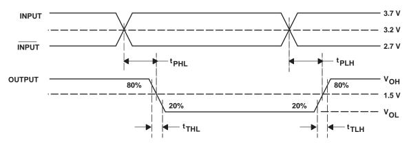
Figure 4. Receiver Propagation Delay Times
