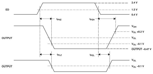
A. NOTE: In the third state, OUTPUT is 0.47 V (minimum) more negative than OUTPUT.
