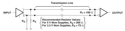
Figure 18. A Recommended pi Load Circuit
