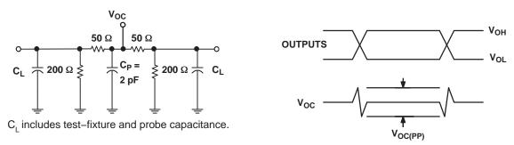
A. NOTE: All input pulses are supplied by a generator having the following characteristics:  $t_r$  or  $t_f$  = 1 ns, pulse repetition rate (PRR) = 0.25 Mbps, pulse width = 500  $\pm$  10 ns.  $C_P$  includes the instrumentation and fixture capacitance within 0,06 m of the D.U.T. The measurement of  $V_{OS(PP)}$  is made on test equipment with a -3 dB bandwidth of at least 1 GHz.
