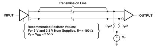
Figure 20. A Recommended PECL-Style Load Circuit
