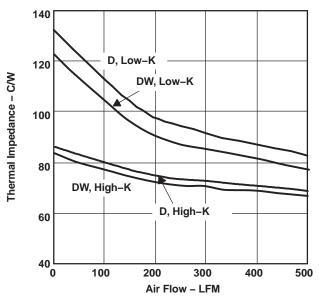
Figure 17. Thermal Impedance vs Air Flow
