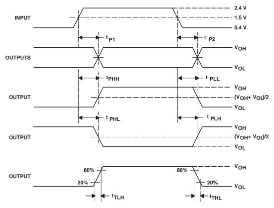
Figure 2. Driver Propagation Delay Times
