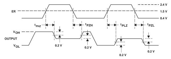
Figure 5. Receiver Enable and Disable Timing
