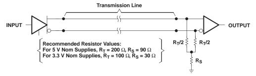
Figure 19. A Recommended Y Load Circuit
