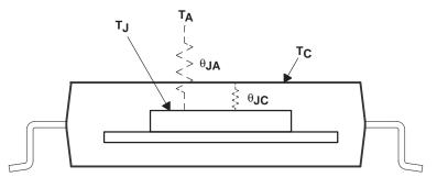
Figure 2. IC Package Thermal Metrics
