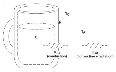
Figure 1. Coffee-Cup Example for Thermal Metrics
