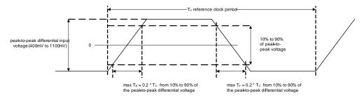
The exception to this is the USB reference clock. In some devices, this clock uses the LJCB buffer. In other devices, it must meet the peak-to-peak voltage limits and the rise and fall time limits shown in Figure 14. The rise time can be no less then 75 ps and no more then 500 ps for the 300 mV(pk-pk) around the center of the differential peak-to-peak voltage.
