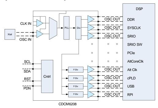
The CDCM6208 incorporates fractional dividers. When assigning fractional divider outputs from the CDCM6208, it will be necessary to verify that the input jitter and performance meet or exceed the requirements for the respective device input (select the correct clock outputs for the proper clock inputs).
