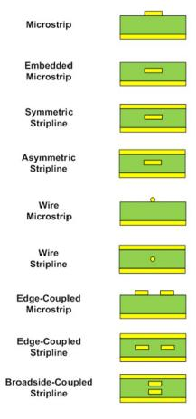
There are multiple impedance calculators available to designers, many of which comprehend these geometries. Two such calculators are available at www.eeweb.com/toolbox/microstrip-impedance/ and at www.technick.net/public/code/.
