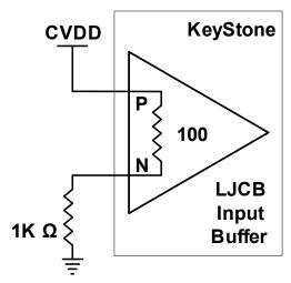
The recommended connections for unused LVDS inputs are shown in Figure 16. The added 1-k $\Omega$  resistors are included to reduce power consumption. The positive terminal should be connected to the DVDD18 power rail.
