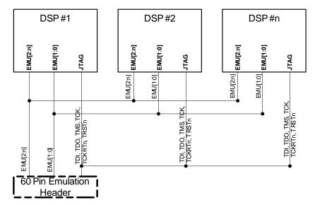
No external pull-up/down resistors are needed because there are internal pull-up/down resistors on all emulation signals.
