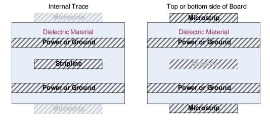
The most obvious difference between these two topologies is the location of the respective net (trace). In a stripline topology (left side) the net or trace is embedded in the PCB and usually between ground or power layers. In the microstrip topology (right side), the net or trace is on an outer layer and adjacent to a power or ground plane.
