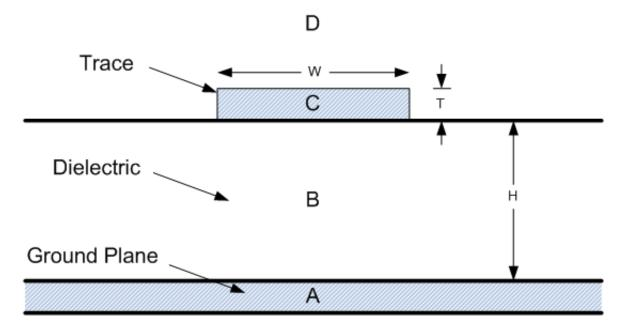
The characteristic impedance of a microstrip transmission line depends on a number of factors including, the width (W) and thickness (T) of the trace (C), and the thickness (H) of dielectric.
