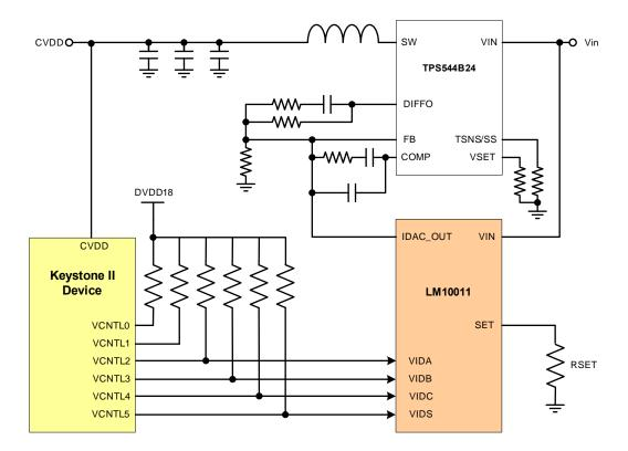
VIDA, VIDB, VIDC, and VIDS are connected to VCNTL2, VCNTL3, VCNTL4, and VCNTL5, respectively. The LM10011 uses a supply voltage in a range from 3 V to 5.5 V, however, the VID inputs are compatible with the 1.8-V logic levels used by the KeyStone II device and no voltage translator is needed. Remember that the VCNTL outputs are open-drain and require a 4.7-k $\Omega$  pull-up resistor to the KeyStone II device DVDD18 rail.
