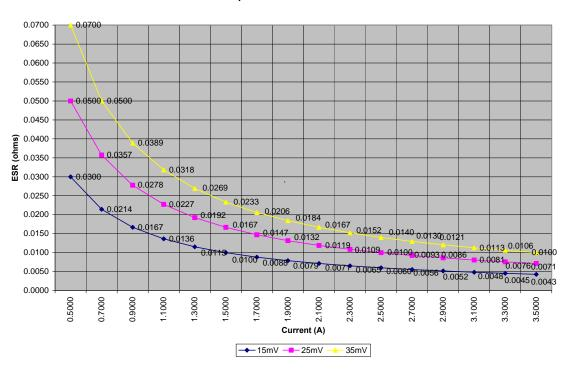
Figure 10 ESR Plot for Delta Current to Tolerance #2
