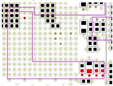
The connections to the ferrite and the local decoupling is highlighted in the lower right and the pin for the KeyStone II device is shown on the upper left. The outline delineates the cut-out on the inner layer creating the small local plane associated with this filtered voltage. The same calculation shown above can be used to calculate the resistivity of the plane.
