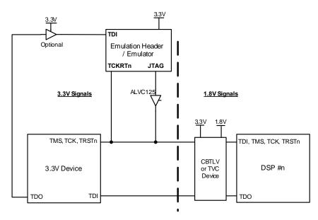
If the trace signals are supported, they may need to have voltage translation as well. Because of the speed of the trace signals, it is recommended that these signals be connected directly to the emulation header.
