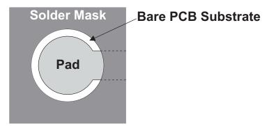
While the size control is dependent on copper etching and is not as accurate as the solder mask defined method, the overall pattern registration is dependent on the copper artwork, which is quite accurate. The trade-off is between accurate dot placement and accurate dot size. NSMD lands are recommended for small-pitch BGA packages because more space is left between the copper lands for signal traces. Dimensioning for the pad and mask are provided in the *Flip Chip BGA Users Guide* (SPRU811).
