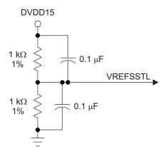
All resistive components must be 1% or better tolerance. The VREFSSTL voltage created by the voltage divider should be routed to the KeyStone II device and the memory components using a trace width of 20 mil or greater. Additional bypass capacitors should be placed next to the connections at the KeyStone II device and the memories.
