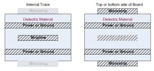
A number of physical and electrical factors govern whether signaling should use microstrip or stripline topology. The key factors determining which topology is used include:
