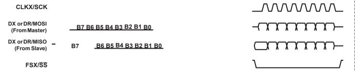
Figure 2. SPI Transfer With CLKSTP = 11 and CLKXP = 0
