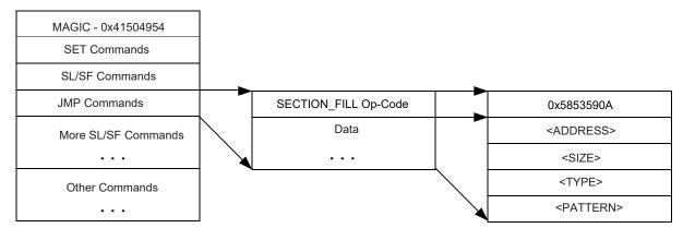
Figure 10. Structure of Section Fill Command
