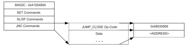
Figure 12. Structure of Jump Close Command
