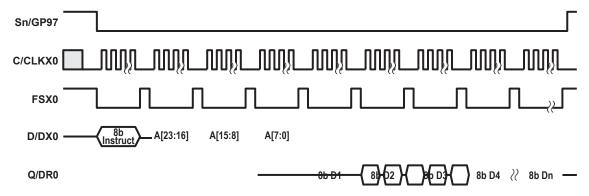
Figure 4. DM643x 24x8 Bit Address SPI Boot
