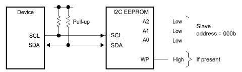
Figure 1. Signal Connections for I2C EEPROM Boot Mode
