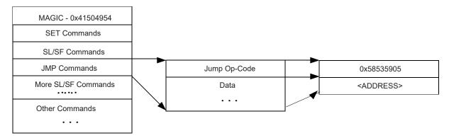
Figure 11. Structure of Jump Command
