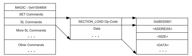
Figure 9. Structure of Section Load Command
