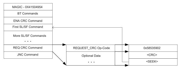
Figure 14. Structure of Request CRC Command
