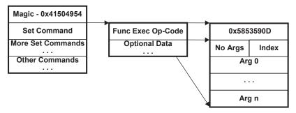
Figure 15. Structure of Function Execute Command
