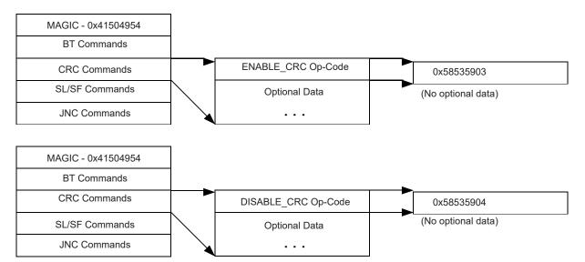
Figure 13. Structure of Enable CRC/Disable CRC Commands
