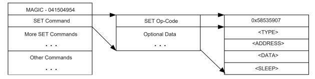
Figure 6. Structure of SET Command
